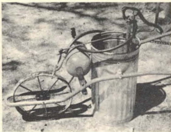
A wheelbarrow type sprayer suitable for spraying tobacco plant beds.
