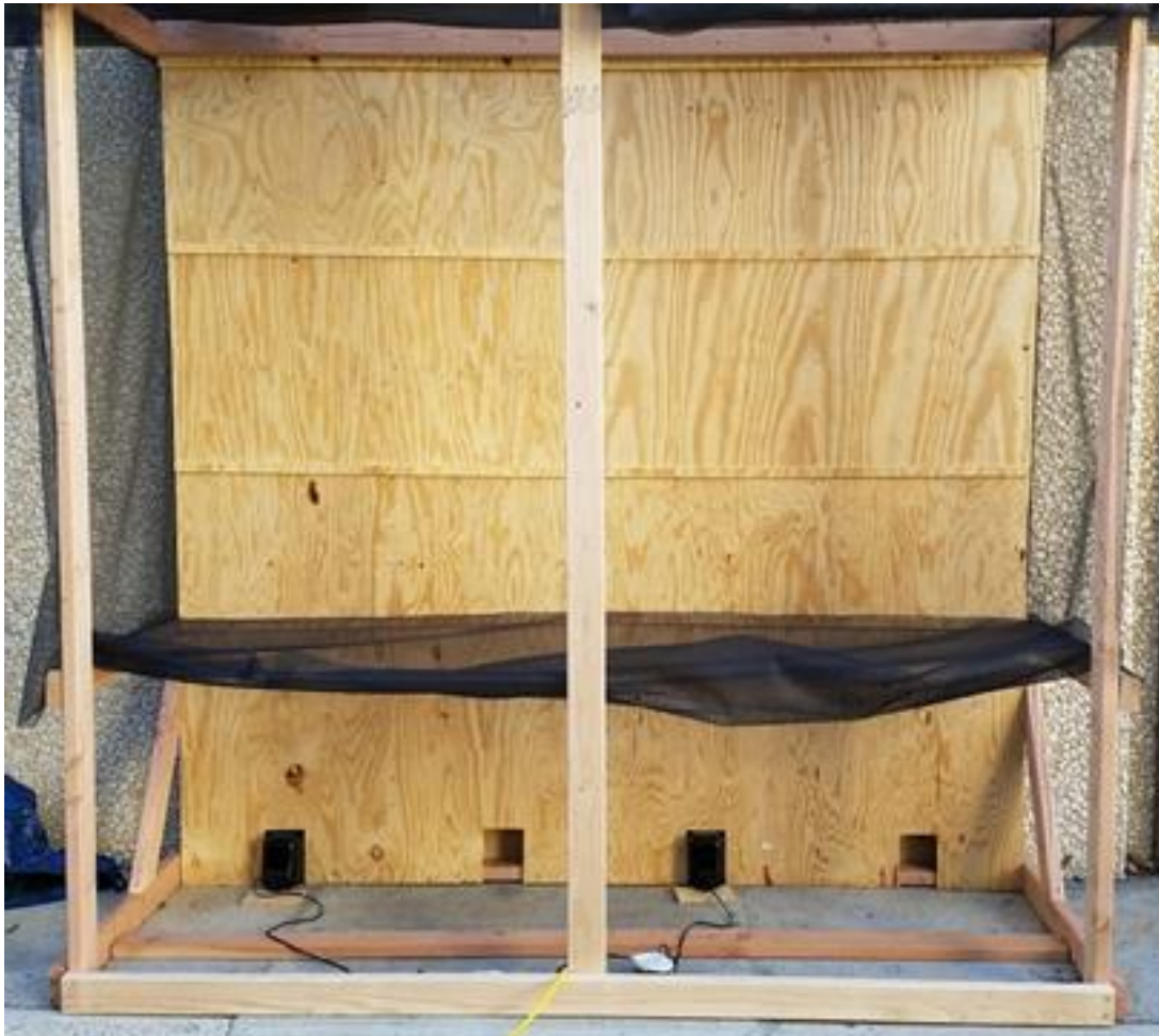
Figure 3.1: Pilot wall panel apparatus with seam cover strips.
