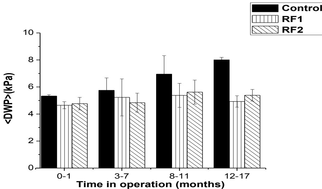
Figure 2.2 Impact of Reverse Flexing (RF) on weighted dynamic wet pressure (DWP) of polyurethane Messner panel diffusers over time in operation
