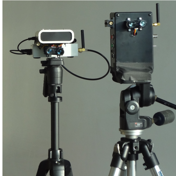
Figure 5.4: Photograph of the lidar instruments. The tripod-mounted instrument on the left contains a Garmin (formerly PulsedLight, Inc.) LIDAR-Lite v2 device, and the instrument on the right contains a Garmin LIDAR-Lite v3 device. Photograph made by the dissertation author.
