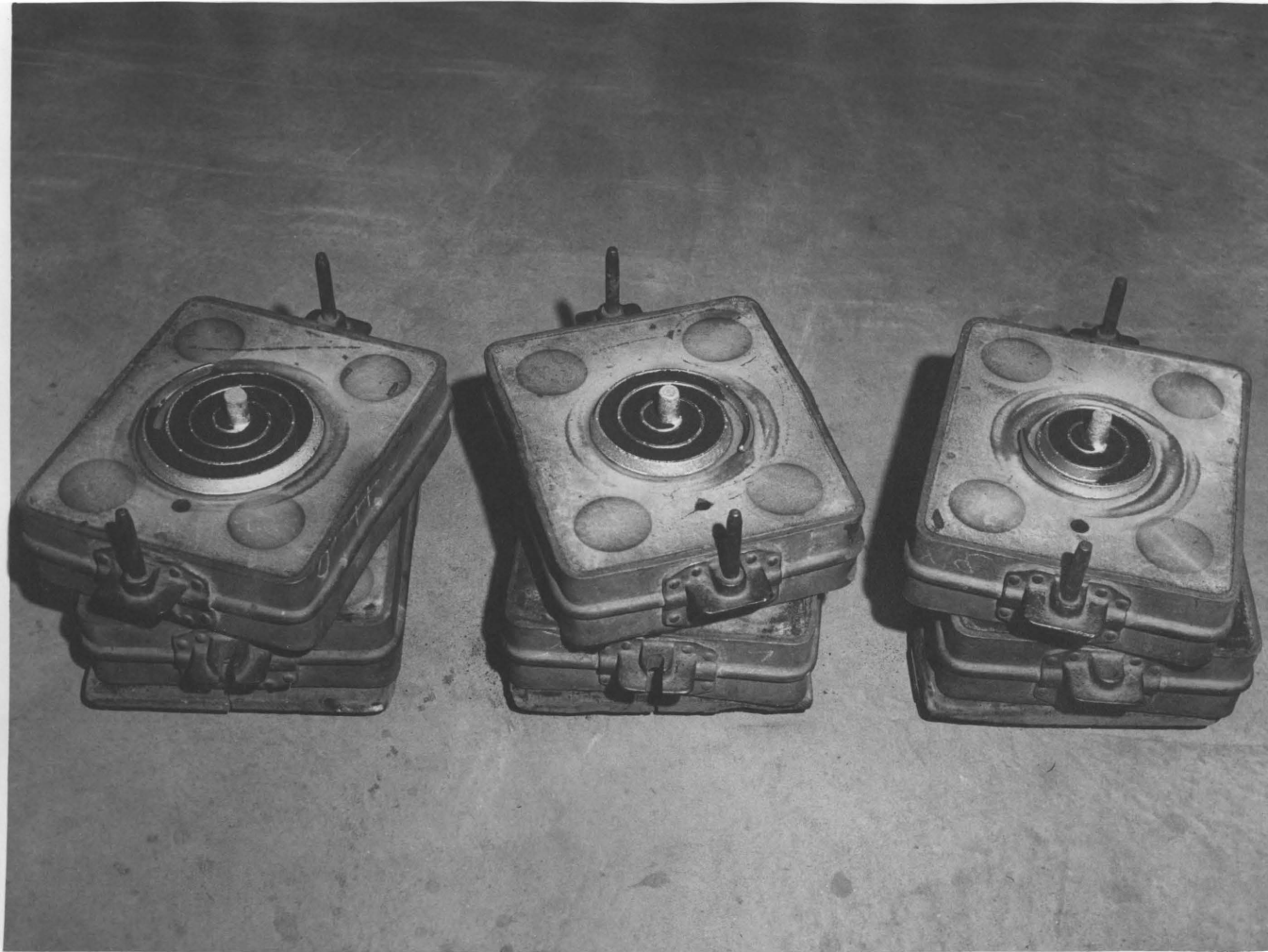
Photograph 6 - Test Molds Poured at 300°F, 200°F, and 100°F Superheat
