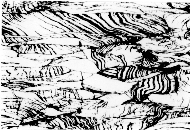
Figure 1. Photomicrograph of HERF 316 stainless steel (200X)
