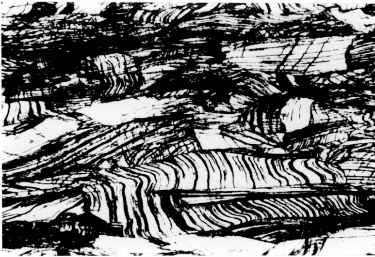
Figure 2. Photomicrograph of S.HERF 316 stainless steel (200X)
