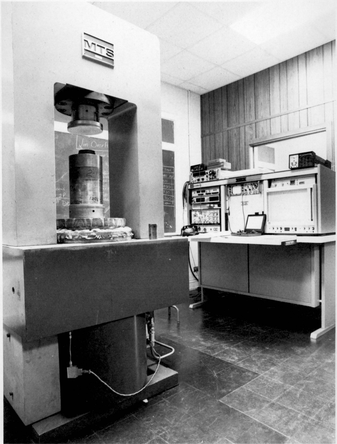
Figure 5.4 MTS Stiff Testing Machine and Control Console
