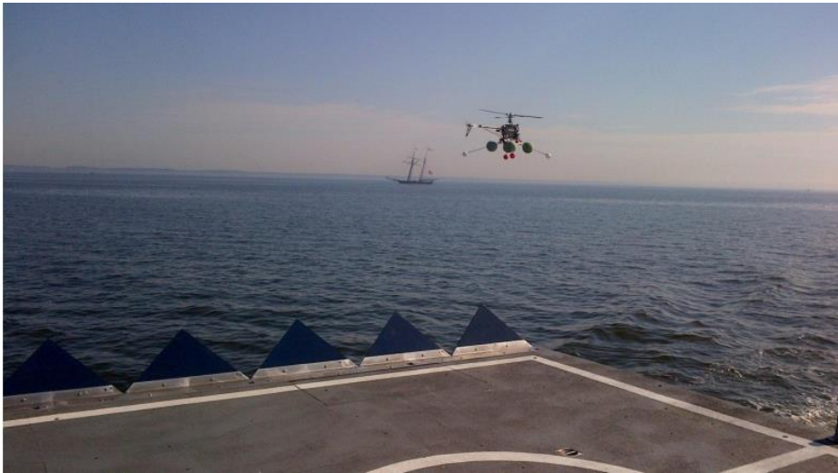
Figure 2.1: Radio controlled instrumented helicopter flying astern of YP676 in the Chesapeake Bay [20].
