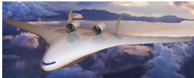
Figure 2.1: Example of boundary layer ingesting aircraft concept ( Image courtesy NASA Langley )
