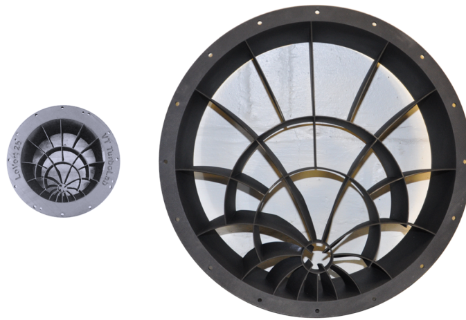
Fig. 2 Small-scale StreamVane (left), and full-scale StreamVane (right) presented to scale.
