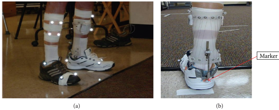
FIGURE 13: Patient wearing the SMA AFO for the motion analysis test.
