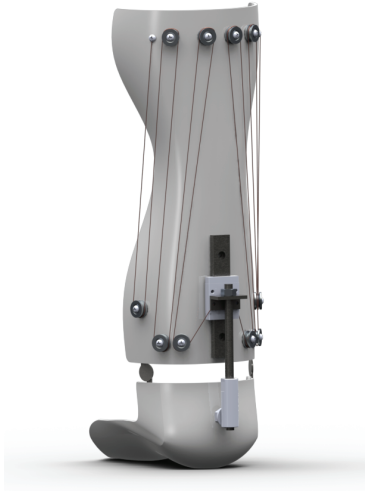
FIGURE 3: The SMA passive AFO CAD design.
