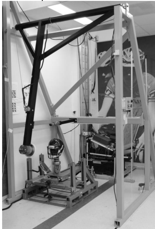
Figure 1: Pendulum impactor used for Adult Football STAR tests.
