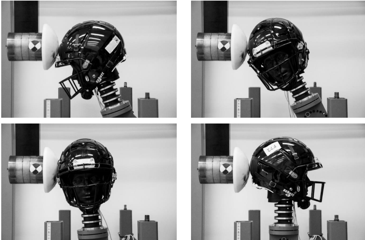
Figure 2: Impact locations clockwise from top left: front, front boss, side, back.
