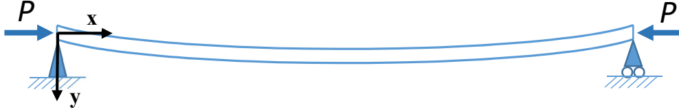
Figure 2-4. Deformed simply supported beam with \phi < 0 .
