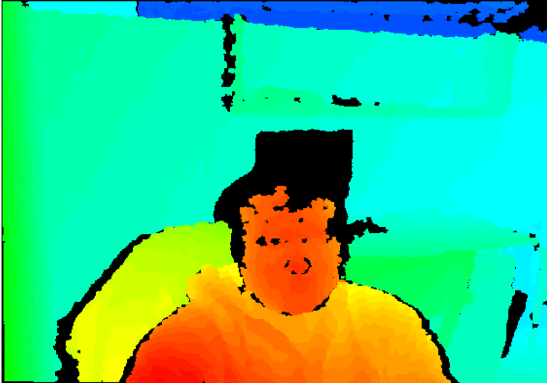
Figure 6. Image. Depth map computed by the depth sensor in an indoor environment.
