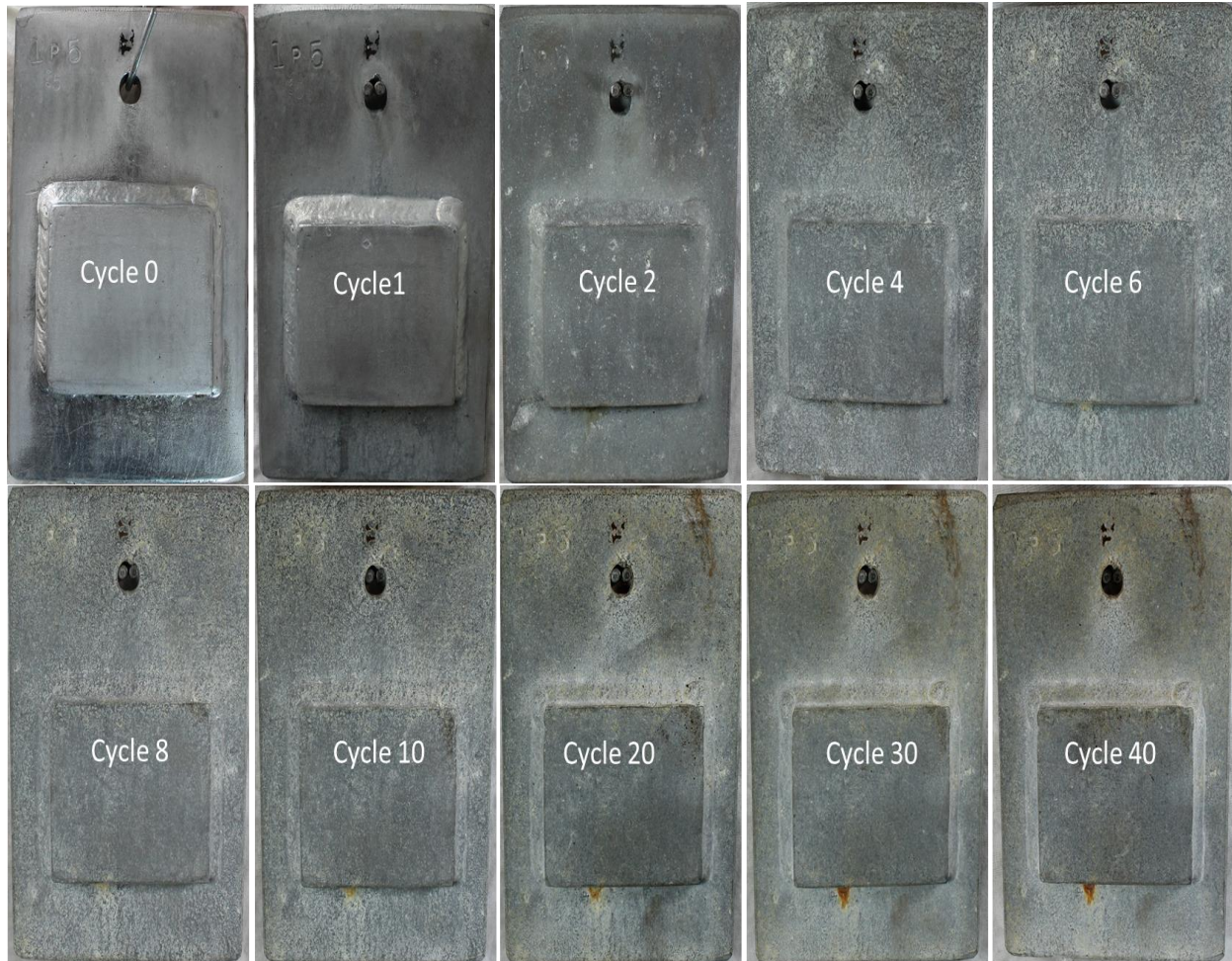
Figure 65: Configuration 5 Specimen 5p5 (not sealed) from 0 to 40 Cycles
