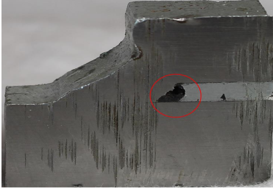
Figure 83: Zinc Coating in the Bottom Interface of the Specimen.
