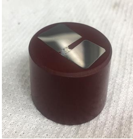
Figure 93: Specimen in a Solid Disc After Heating the Powder
