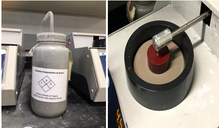
Figure 97: Aluminum Suspension (left) and a Sample in Process (right)
