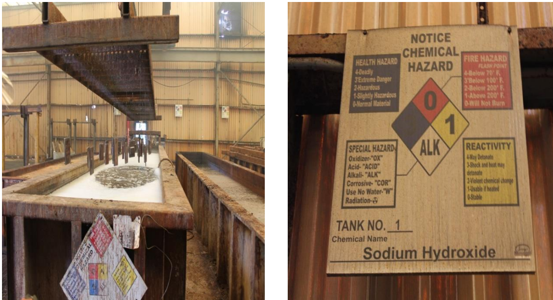
Figure 36: Degreasing Bath with the Chemical Composition
