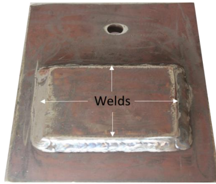
Figure 22: Configuration 1 (welded in all sides)
