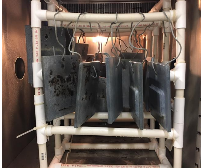
Figure 31: Steel Specimens Hung on PVC Pipes Inside the Chamber
