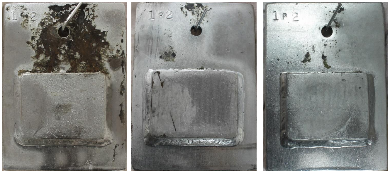
Figure 48: Configuration 2 (open edge on top, no sealants 1p2, 4p2, 5p2)
