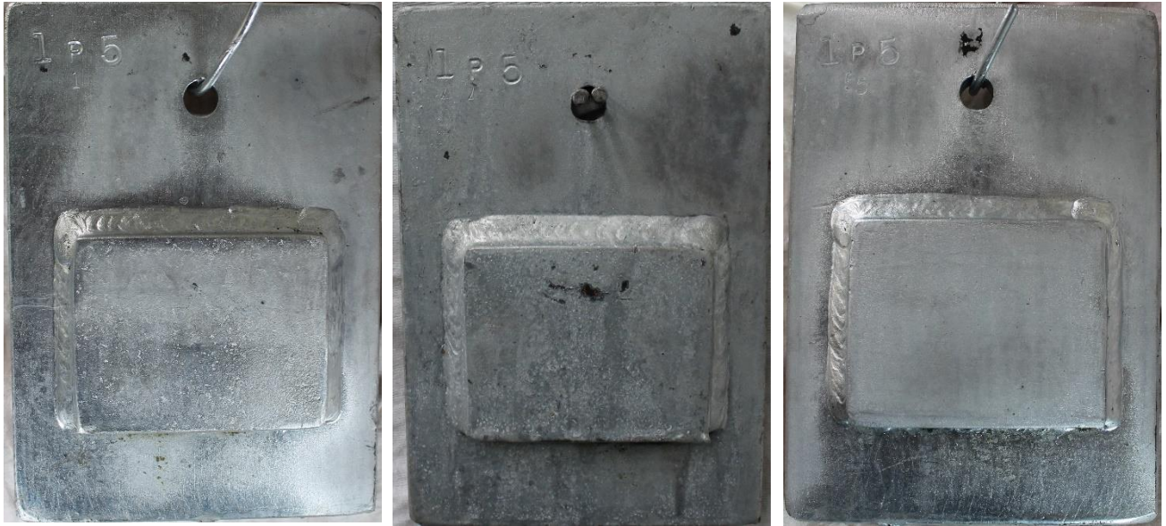
Figure 52: Configuration 5 (open edge on bottom, no sealants 1p5, 4p5, 5p5)
