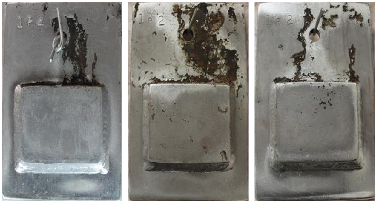
Figure 50: Configuration 2 (GE Silicone Sealant, 2p2, 6p2, 7p2)
