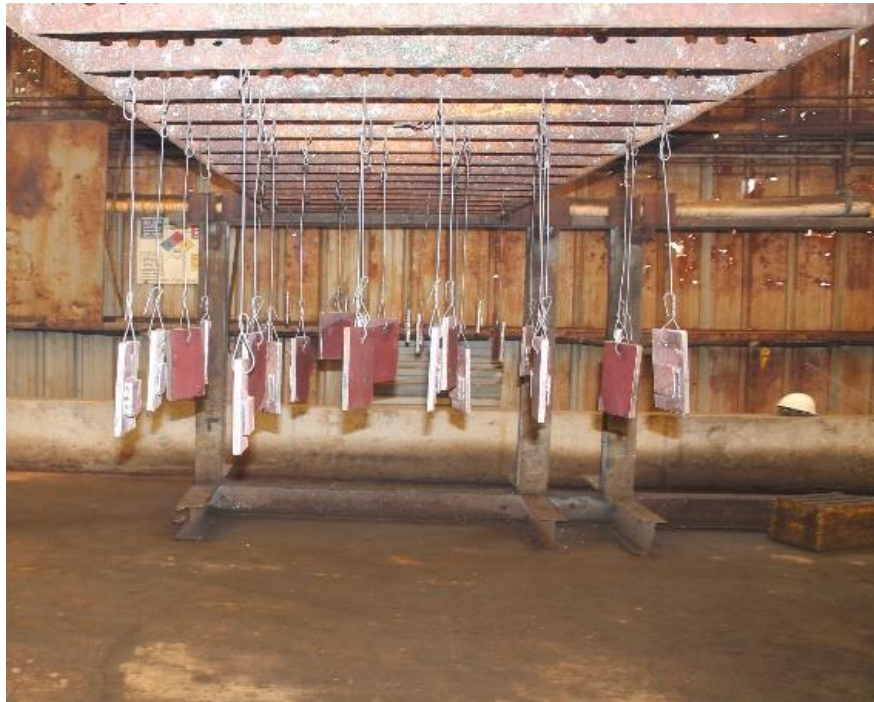
Figure 35: Steel Specimens Hung with a Moveable Crane
