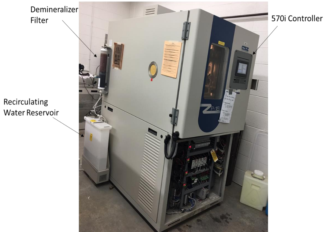
Figure 87: ZP-16 Chamber with Various Components
