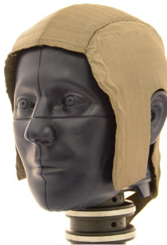
Figure 3: Medium NOCSAE headform with custom pressure sensor array. The pressure sensor array consists of 502 capacitive pressure sensors.
