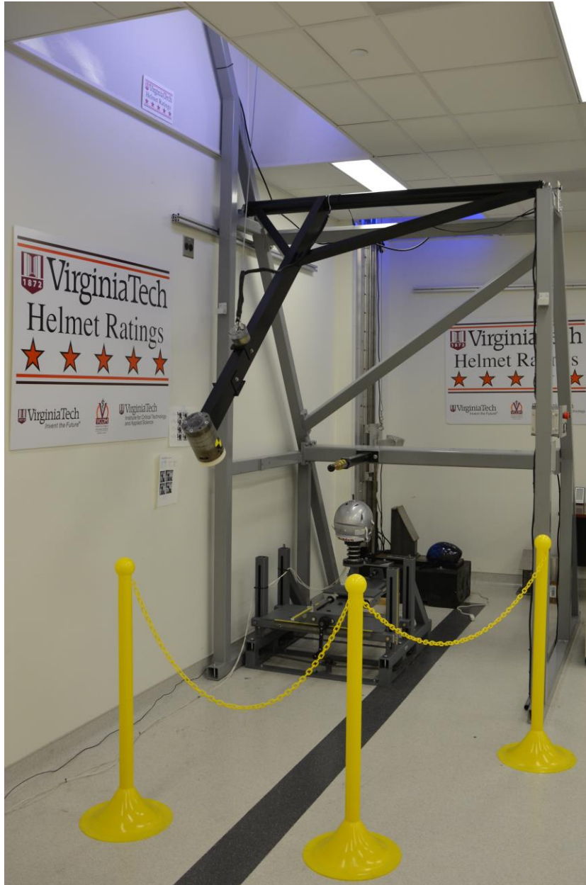
Figure 8: Pendulum impactor used to test helmets. The impactor face at the end of the pendulum arm impacts a helmet on a NOCSAE headform mounted to a Hybrid III neck. The headform-neck assembly is mounted to a 5 DOF linear slide table.
