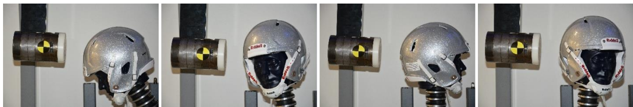
Figure 1: Pendulum impactor impacting helmet in (left to right) front, front boss, rear, and rear boss impact locations.
