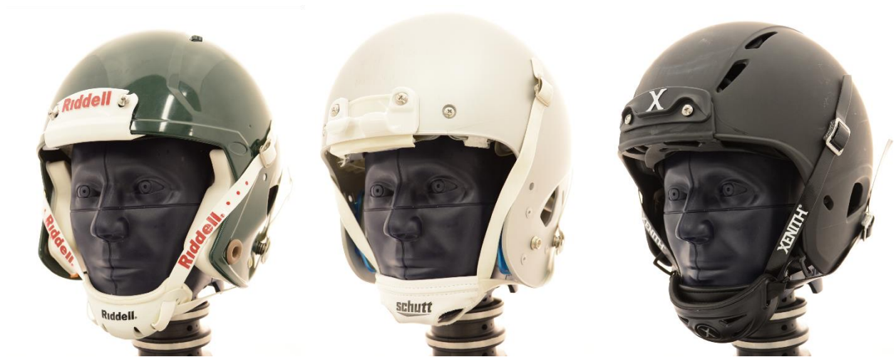
Figure 2: Medium NOCSAE headform with (left to right) Riddell Speed, Schutt Air XP Pro VTD, and Xenith Epic.
