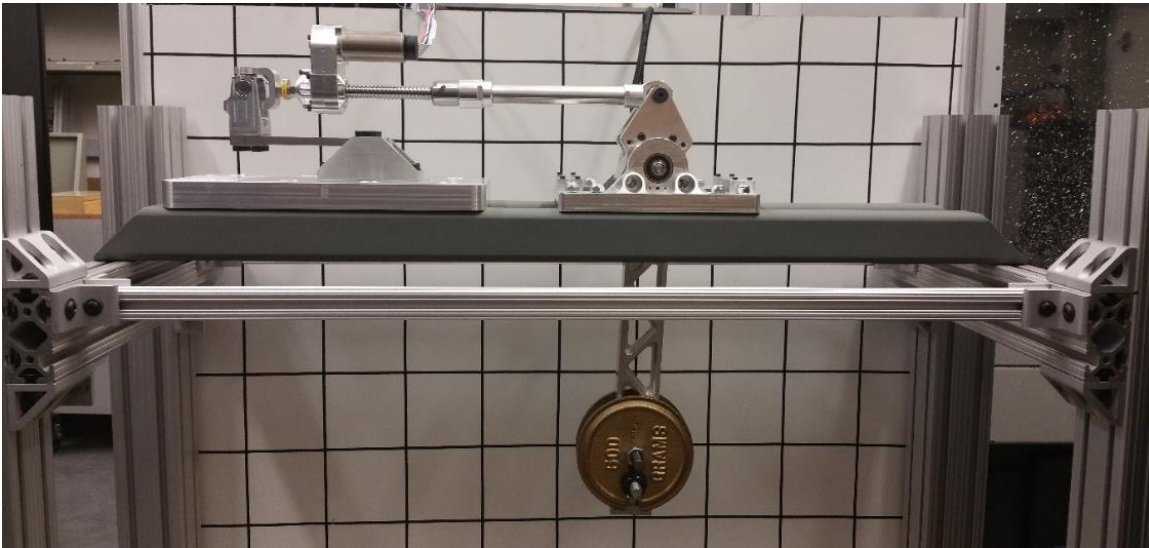
Figure 67: Custom Actuator Test Stand with MKIII Lite Mounted
