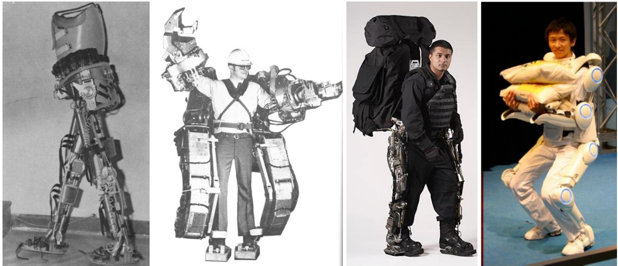
Figure 1: Mihailo Pupin Exoskeleton [15], Hardiman [16], BLEEX [1], HAL-5 [17]
