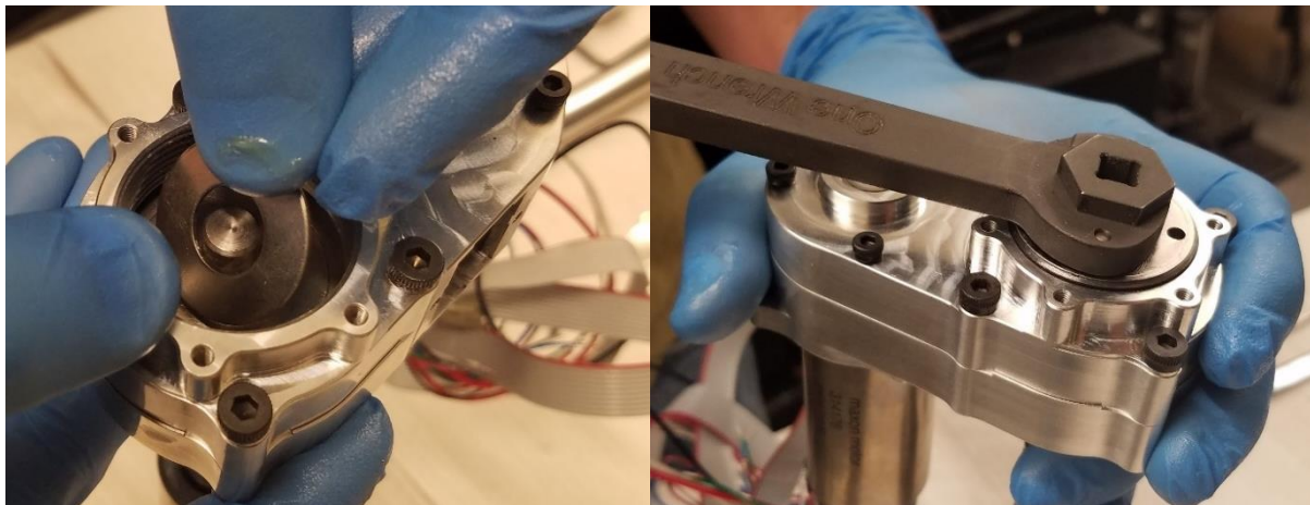
Figure 49: Installation of Bearing Components (Left) and Thrust Nut (Right)
