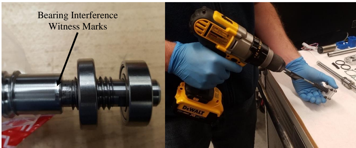
Figure 63: Ball Screw Lower Bearing Fitment Issues (Left) Honing of Inner Race (Right)
