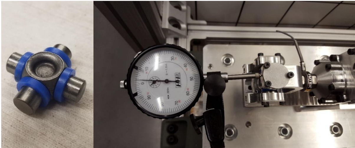
Figure 64: Significant Play Found In U-Joint Trunnion and Bearing
