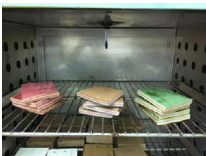
Sample of skateboards in an oven being tested for moisture content and specific gravity.
