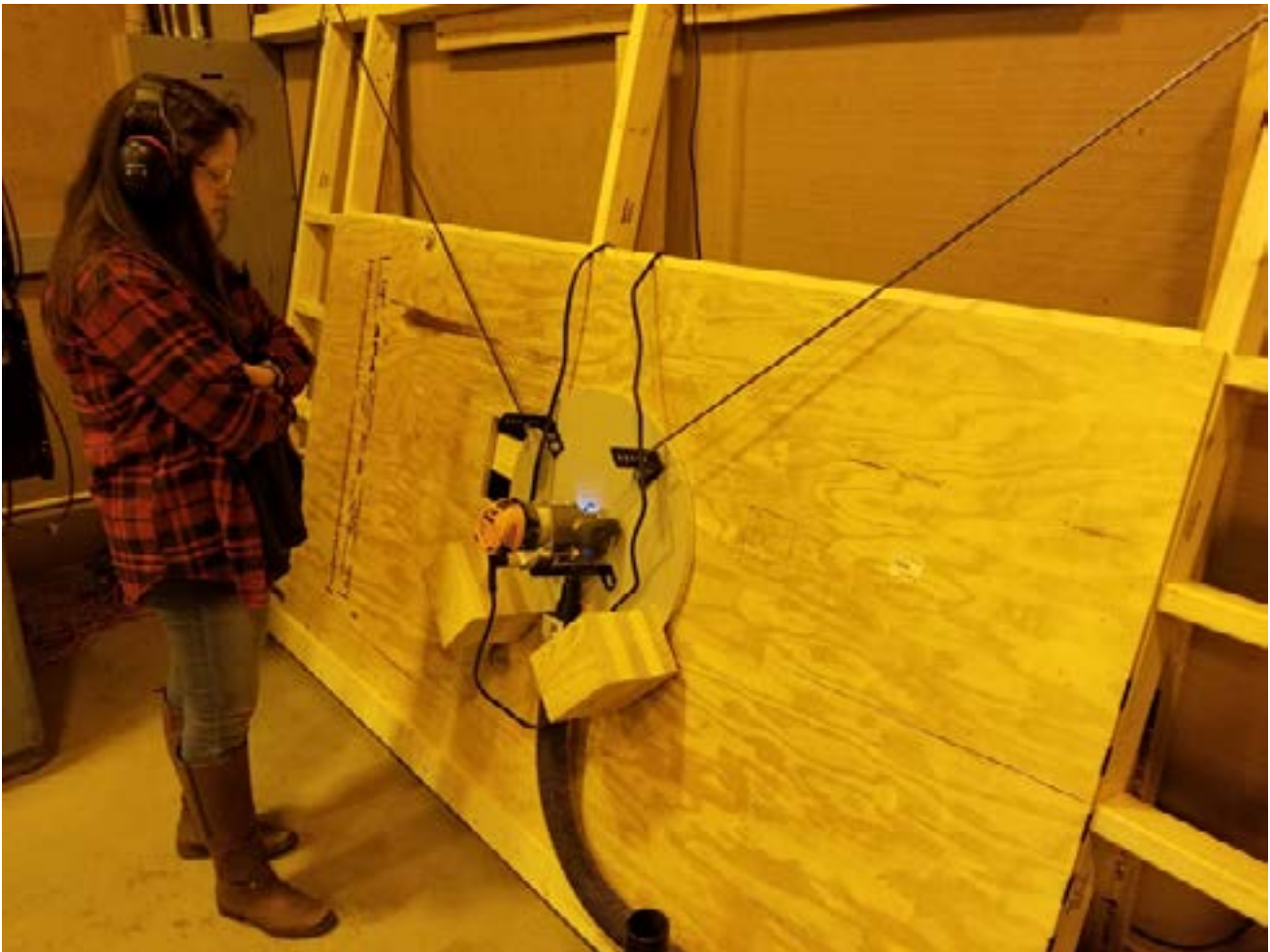
Kerrigan Strong observes the Maslow CNC machine in operation.
