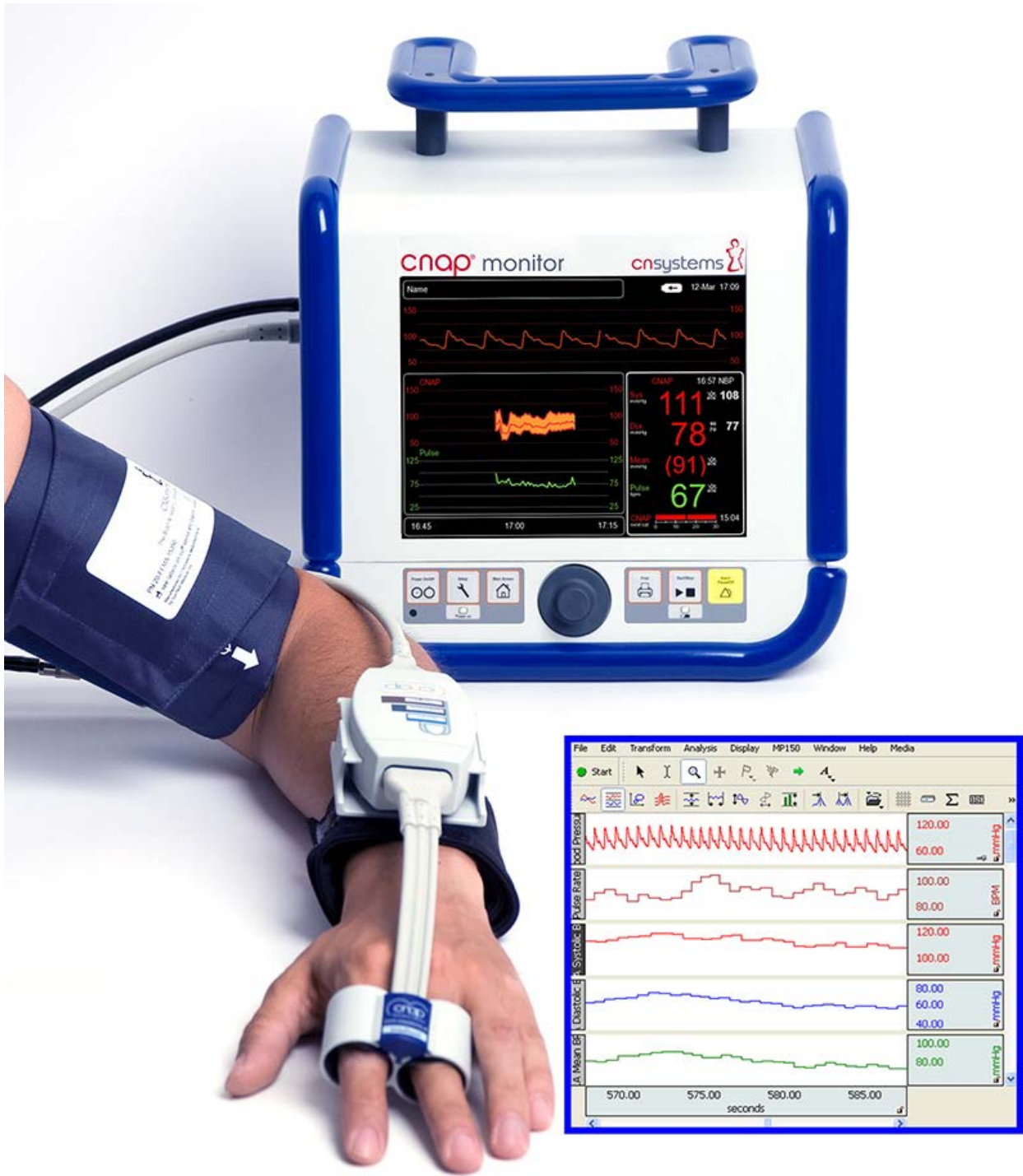
The above device monitors blood pressure and pulse rate. ( https://www.biopac.com/wp-content/uploads/NIBP100D_V3.5_incl_setup_AcqKnowledge_8001.png )
