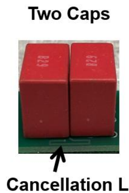
Fig. 4.32 ESL cancellation implementation into PCB
