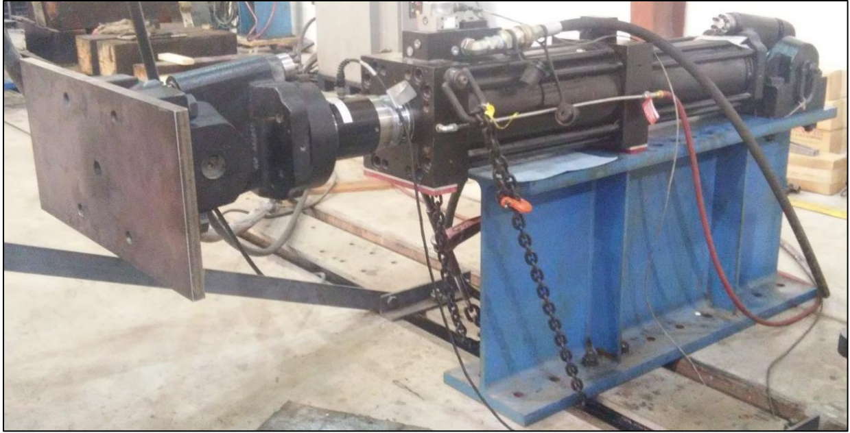
Figure 48: 110 kip horizontal actuator
