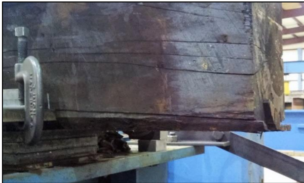
Figure 57: Parallel shear failure of the dap
