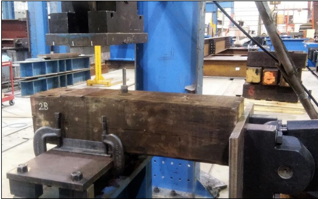
Figure 53: L3x3x1/2 angles clamped using bridge clamps to prevent tie movement
