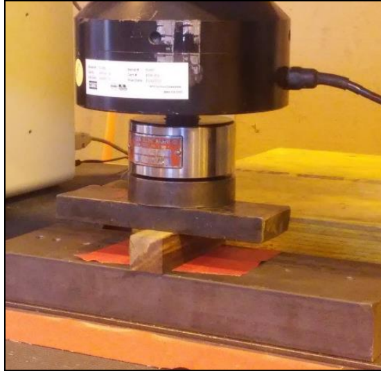
Figure 32: Compressive testing perpendicular to grain
