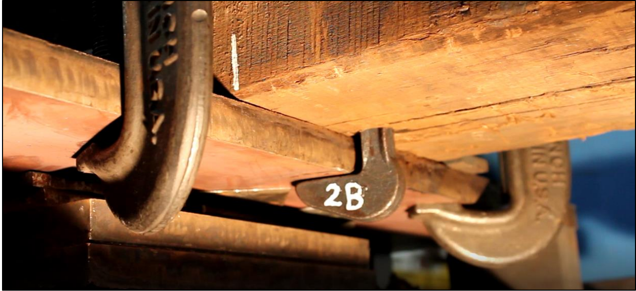
Figure 51: Round body hook bolt attached to 30" x 14" steel plate
