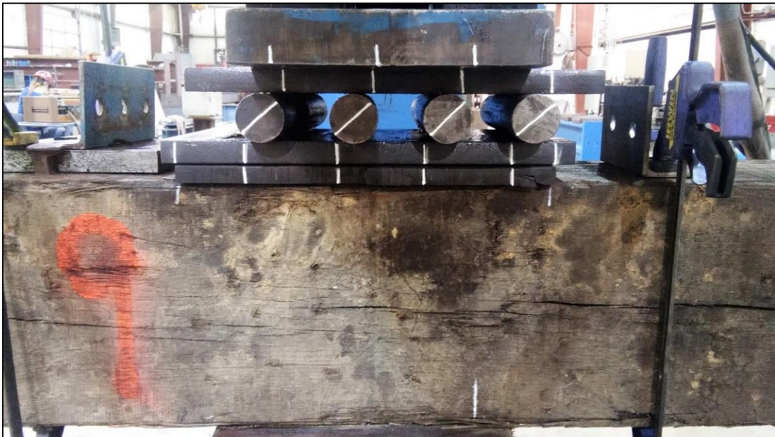
Figure 65: Tie, steel plates, rollers and bearing pads after testing
