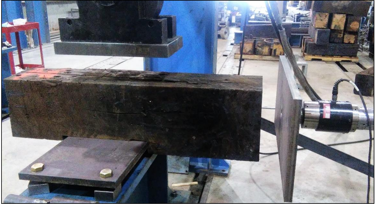
Figure 56: Dapped tie sample prior to testing
