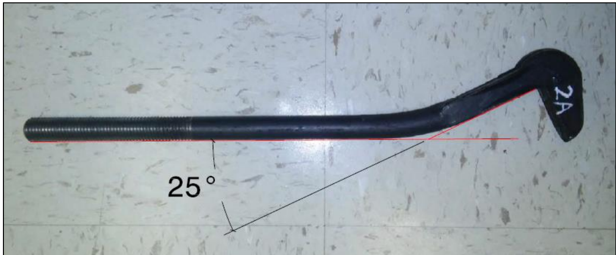
Figure 98: Curvature in a deformed Lewis Forged hook bolt
