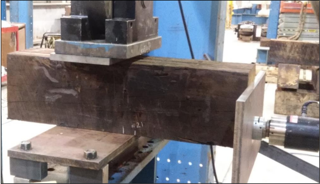
Figure 47: Displaced tie and greased steel plate after friction testing
