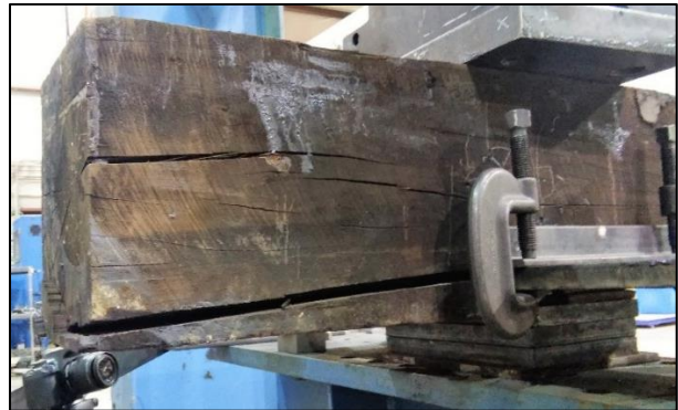
Figure 58: Shear failure of the dap (other side)
