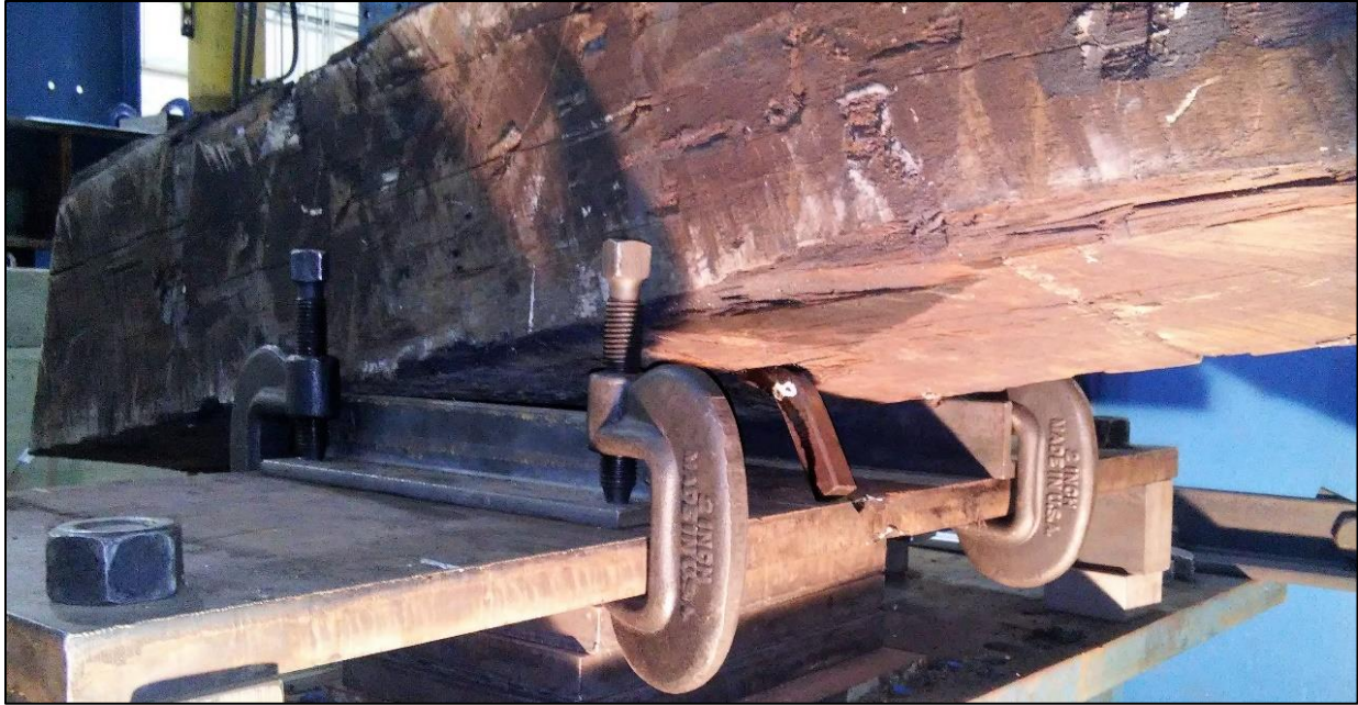
Figure 85: Tie uplift with fastener climbing over the steel plate
