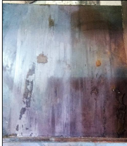
Figure 73: Steel plate after lateral push tests on Tie 5
