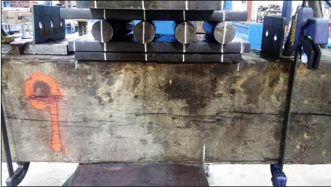
Figure 64: Tie, steel plates, rollers and bearing pads before testing
