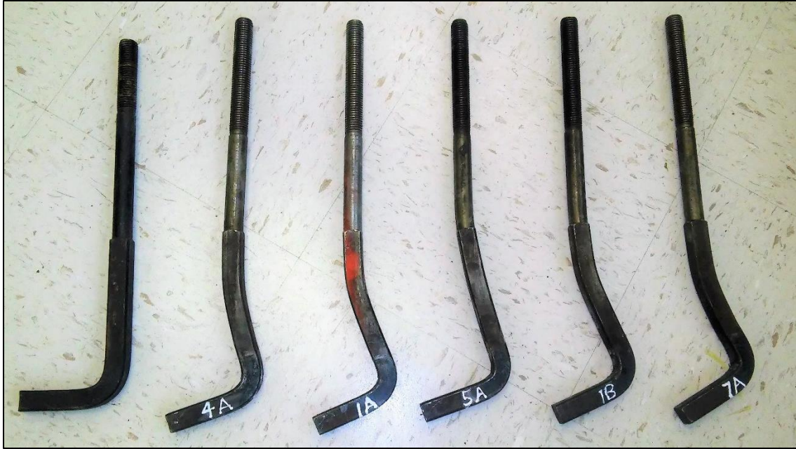
Figure 88: Deformed square body hook bolts after testing
