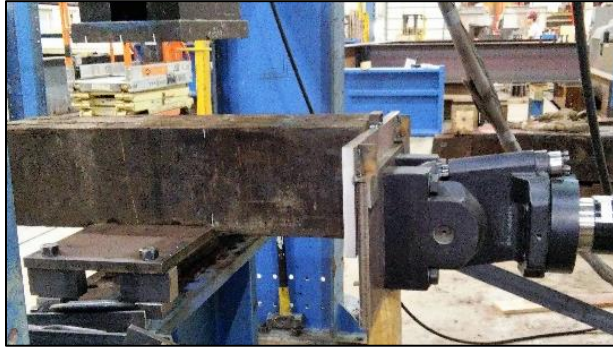
Figure 59: Loading the undapped portion of the tie
