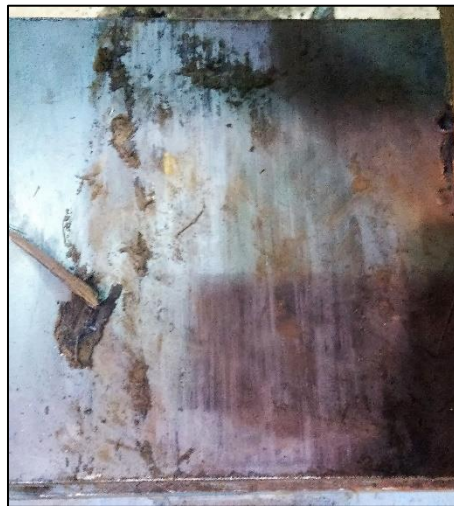
Figure 75: Steel plate after lateral push tests on Tie 8
