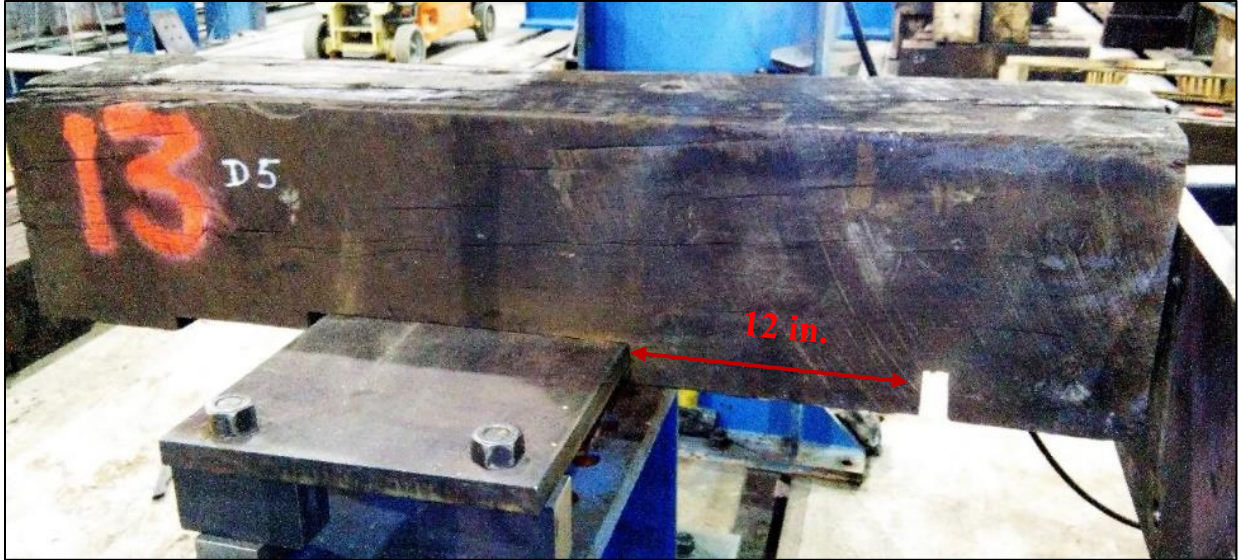
Figure 61: Dapped tie with a 1 inch thick notch
