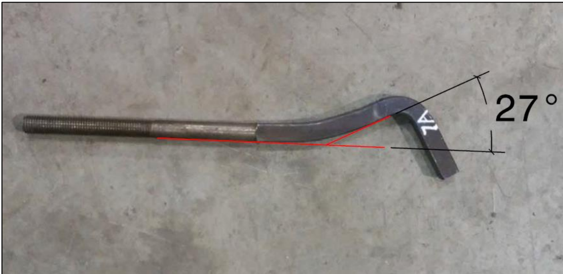
Figure 89: Curvature in a deformed Square body hook bolt
