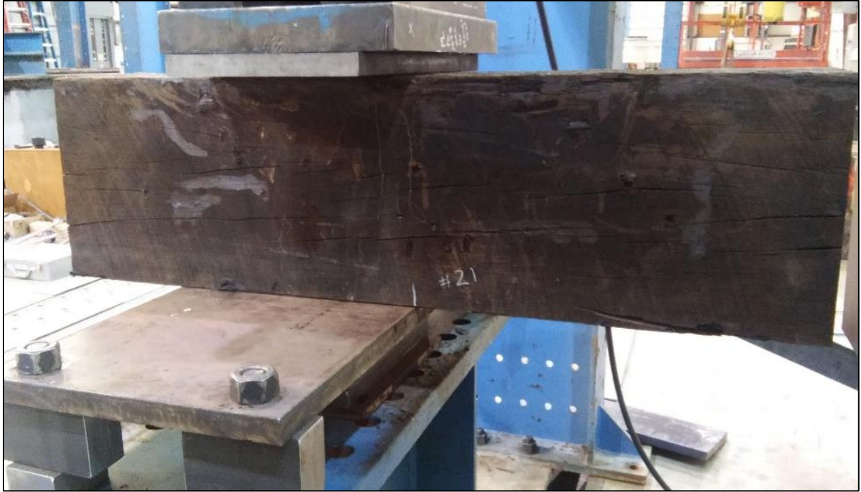
Figure 46: Steel plate with Teflon grease
