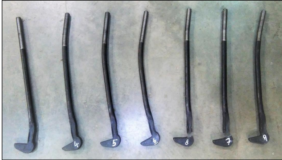
Figure 106: Failed Quikset Anchors after testing
