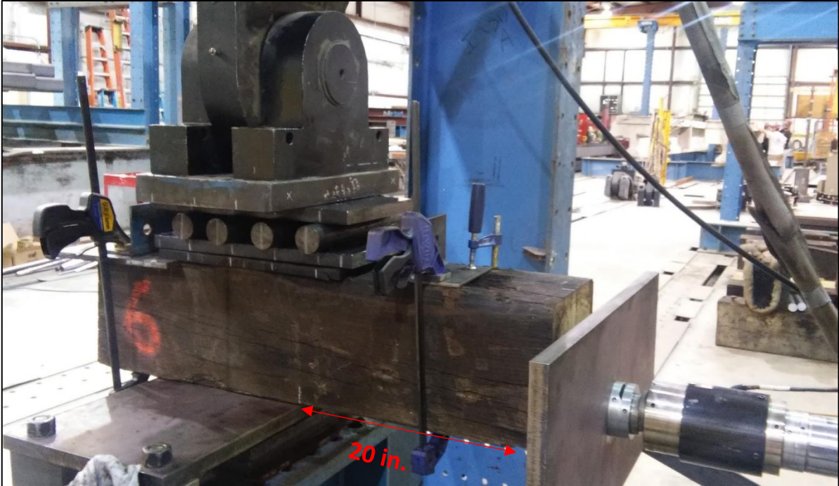
Figure 44: Undamped tie without a fastener
