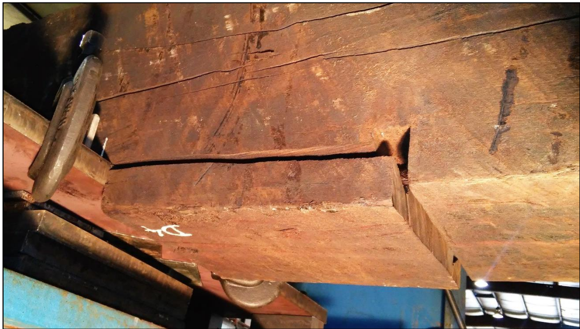
Figure 112: Dap shear failure in tie specimen D4
