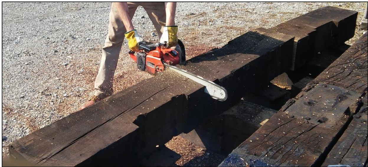
Figure 39: Tie samples were cut with a chainsaw
