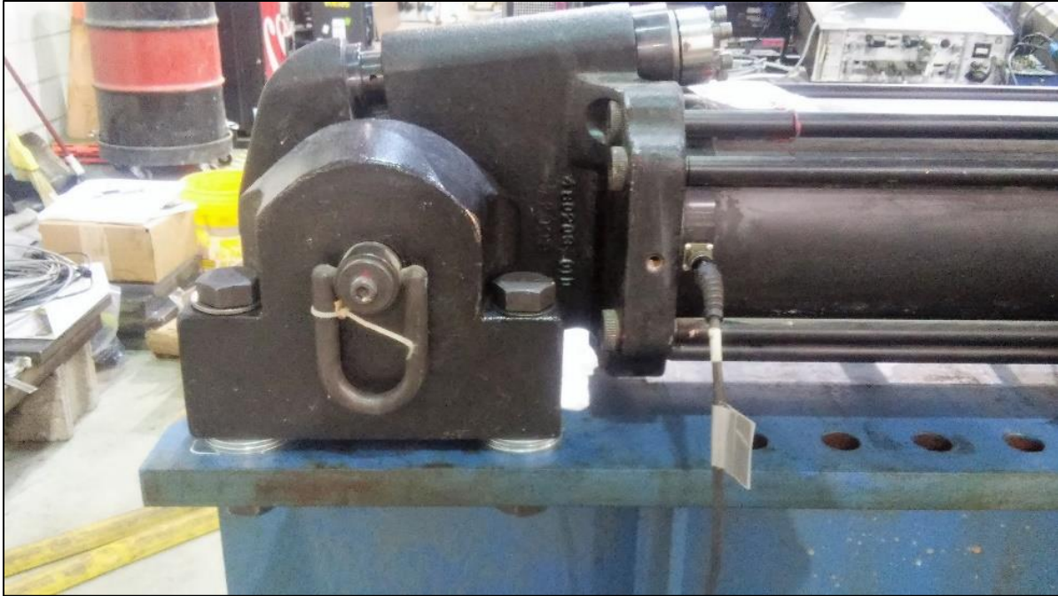
Figure 49: 110 kip actuator raised by washers
