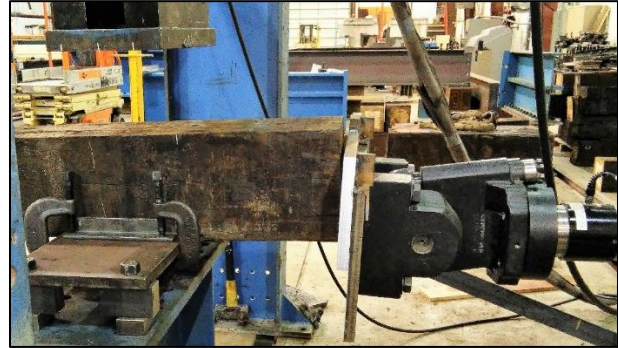
Figure 60: Tie lifting up during loading
