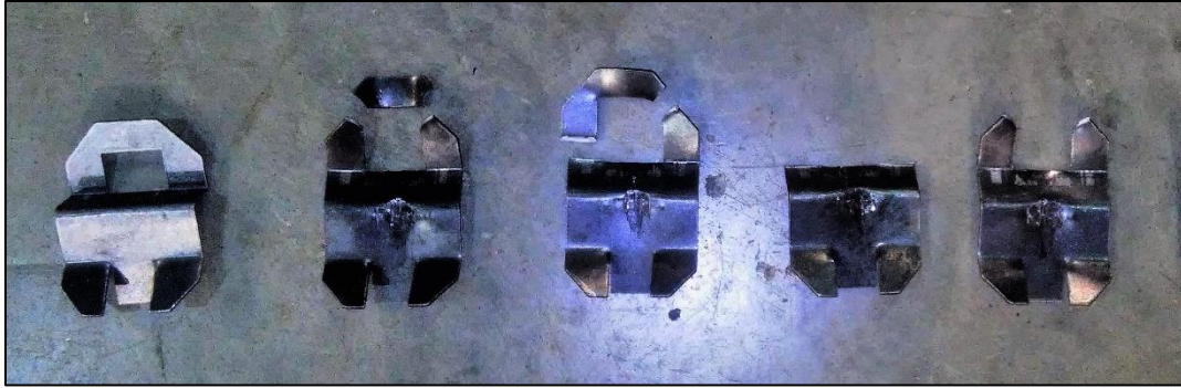
Figure 105: Failed Quikset Anchor lock plates
