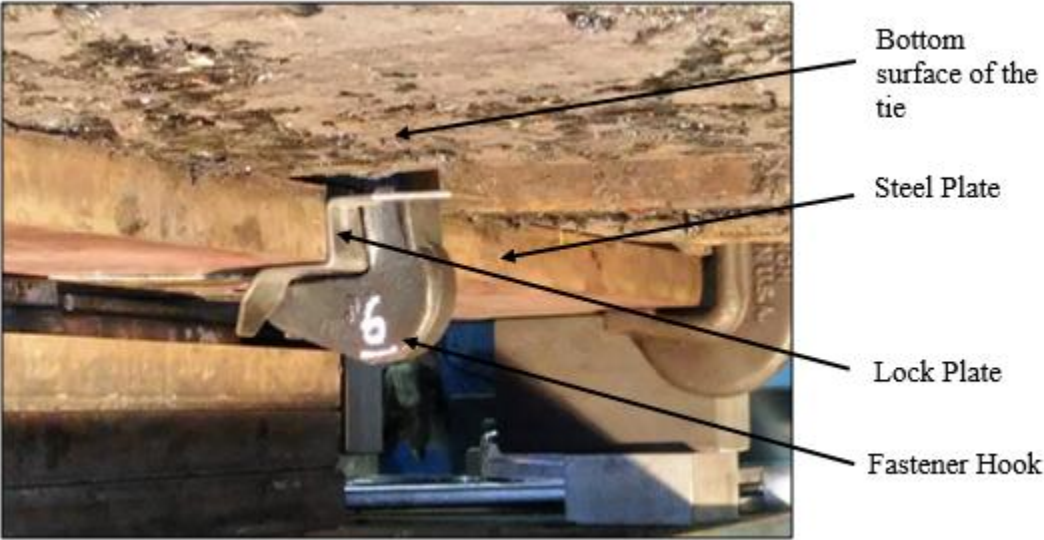
Figure 103: Quikset Anchor before testing
