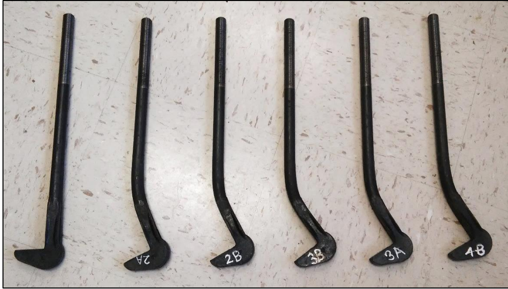
Figure 97: Deformed Lewis Forged hook bolts after testing
