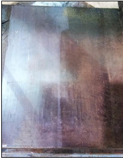
Figure 79: Steel plate after lateral push tests on Tie 9
