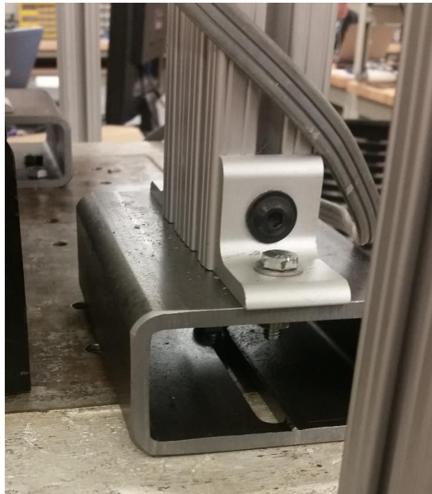
Figure 28: Tubes were bolted to table to allow flexibility for mounting method in this particular experiment
