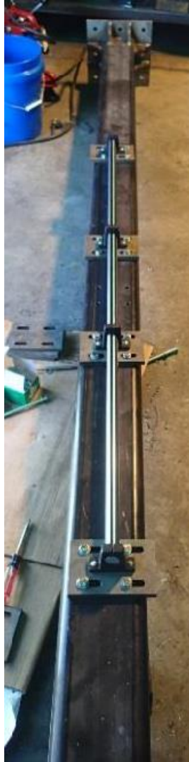
Figure 15: Single support beam with guide rail attached
