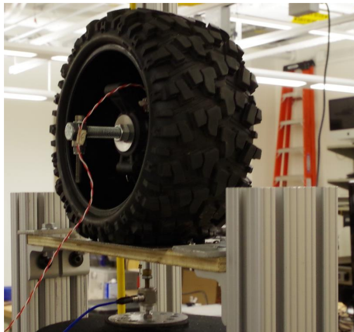
Figure 93: Tire subsystem being excited using the wire setup
