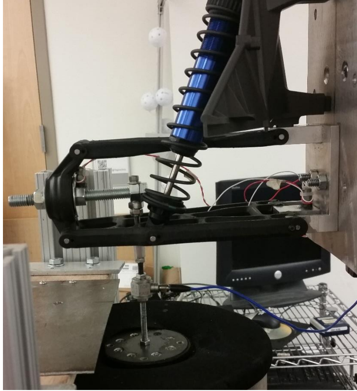
Figure 95: Test configuration for the suspension subsystem by itself
