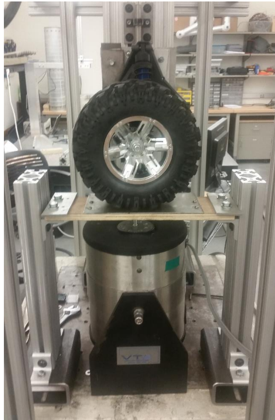
Figure 29: 1530 sized extrusions supply a stiff base along with adjustability
