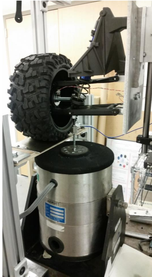
Figure 75: Test setup for excitation directly to unsprung mass
