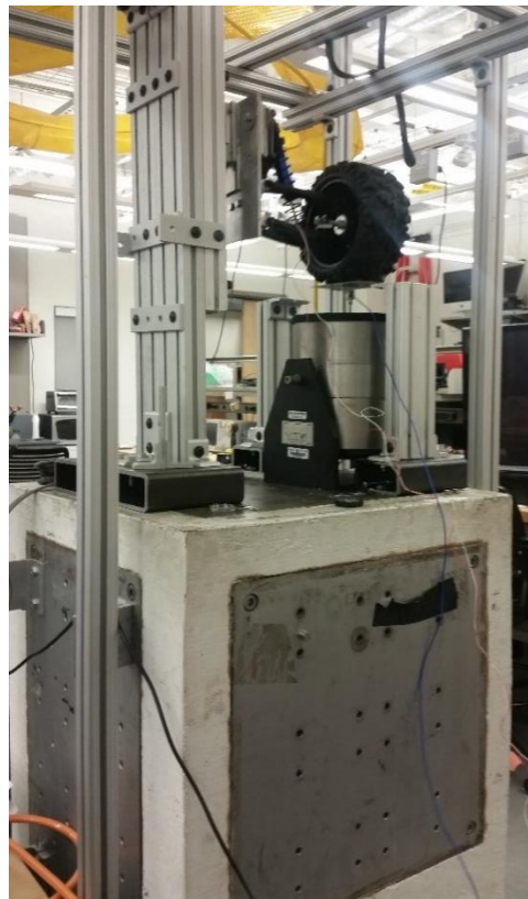
Figure 25: Test stand in VAST laboratory with small-scale quarter car rig attached
