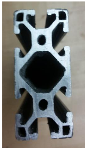
Figure 27: Cross section of a 1530 - Lite aluminum 80/20 extrusion
