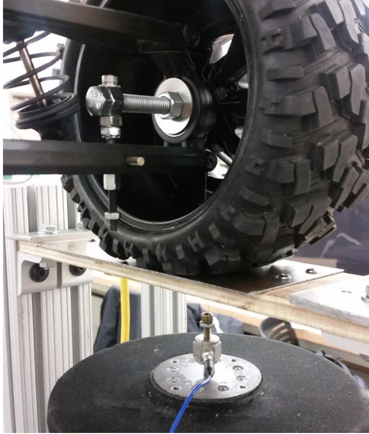
Figure 83: A steel wire is attached directly to the wheel hub and down to the load cell through a small hole in the tire and support surface.
