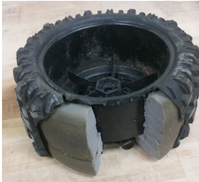
Figure 20: Construction of a typical tire for the test vehicle
