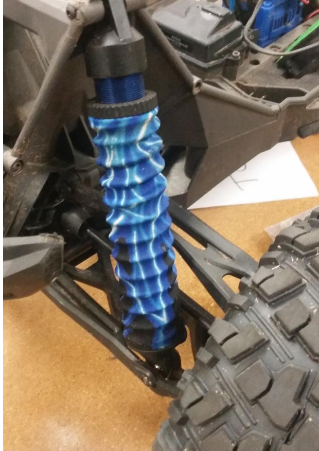
Figure 24: Independent suspension system on the scaled test vehicle
