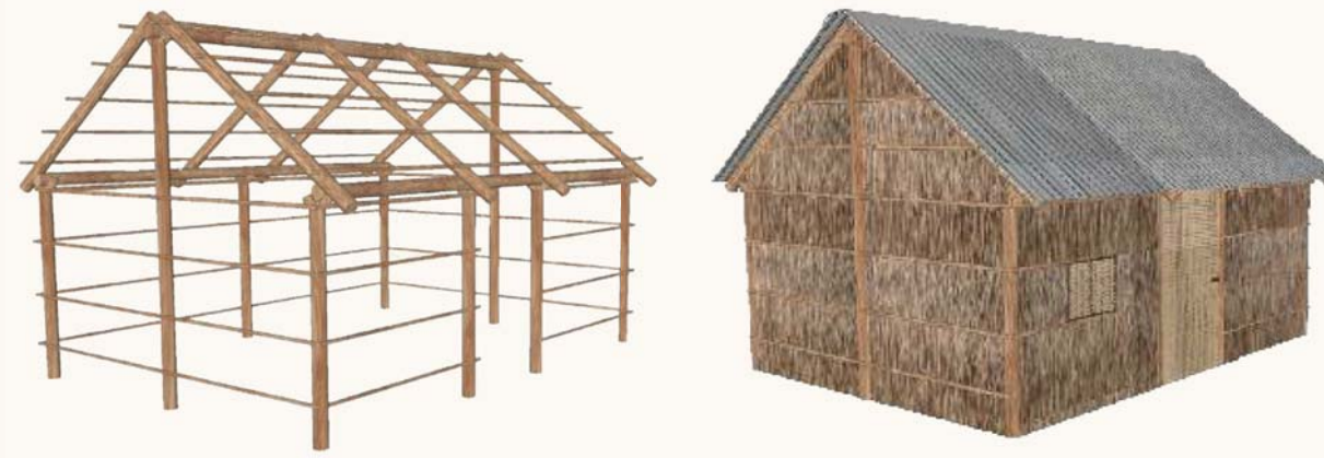
Figure 14_ Wooden gable frame shelter [14]
