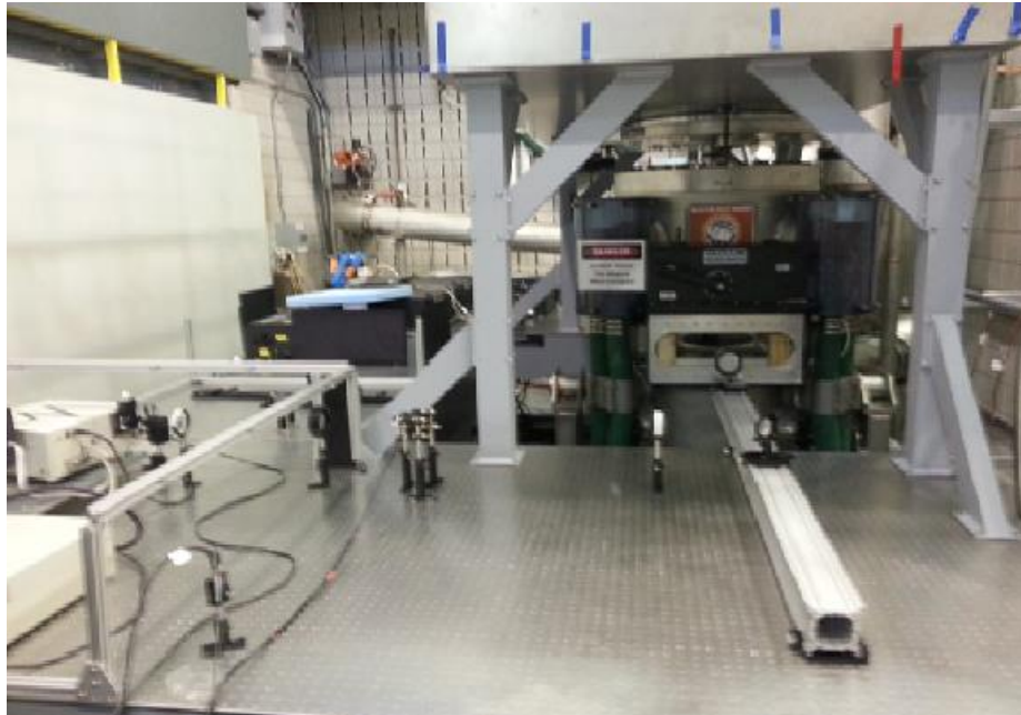
Figure 1.5: The set up used for the MCD measurements. The Split-Florida Helix magnet has optical windows, which preserve the polarization of light, and can provide magnetic fields of upto 31 T.
