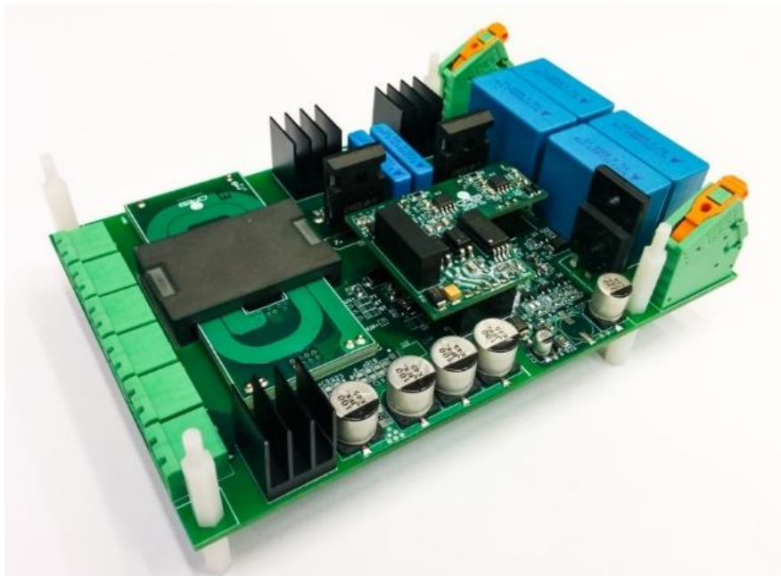
Figure 5-35 Auxiliary power supply prototype
