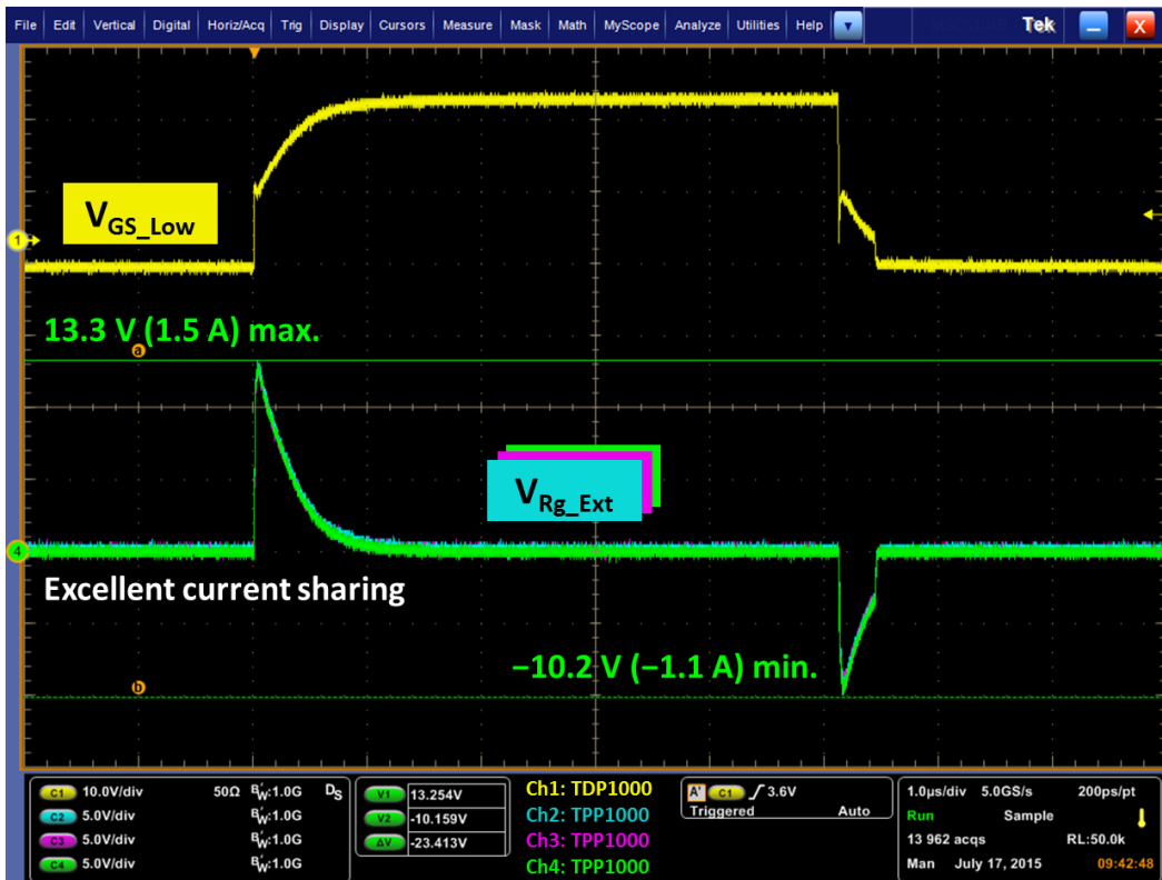
Figure 5-21 Current sharing of three paralleled current boosters
