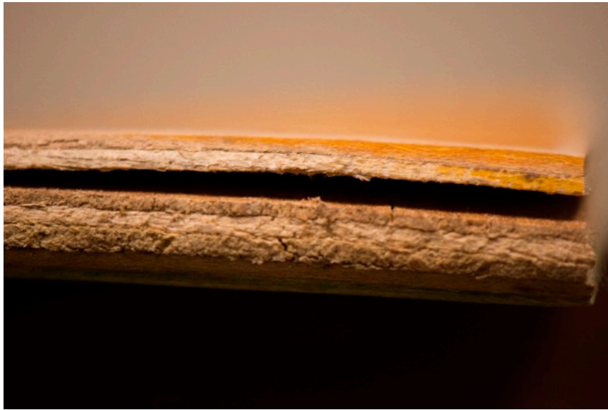
Figure 16. Face wise view of sample 4 showing delamination after soak/dry moisture durability test (ANSI/HVPA EF 2009 [4]).
