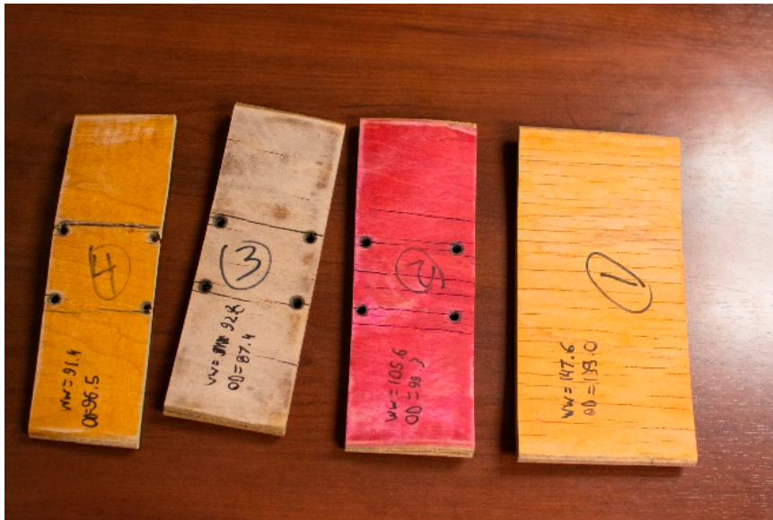
Figure 11. Top view of samples after soak/dry moisture durability test (ANSI/HVPA EF 2009 [4]).
