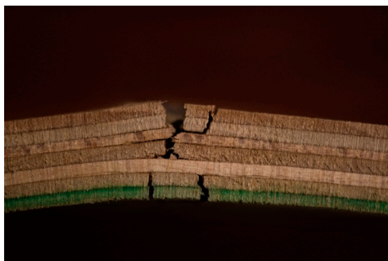
Figure 20. Cross Section View Showing Four Layer Split in Sample 1.
