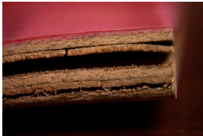
Figure 14. Face wise close up view of sample 2 showing delamination after soak/dry moisture durability test (ANSI/HVPA EF 2009 [4]).
