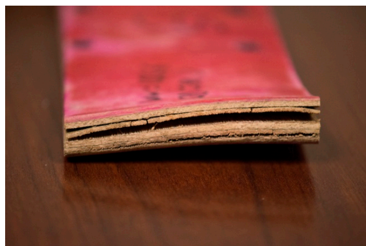
Figure 15. Face wise wide view of sample 2 showing delamination after soak/dry moisture durability test (ANSI/HVPA EF 2009 [4]).
