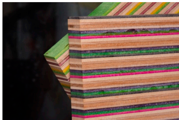
Figure 5. Composite Panels made by cutting skateboard decks into strips and gluing together.
