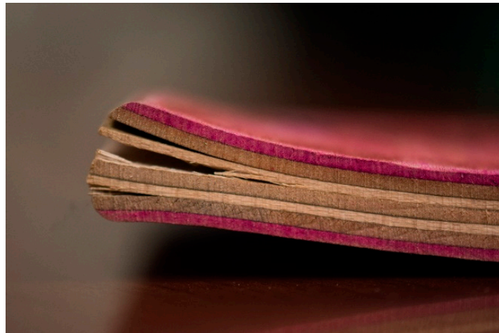
Figure 13. Cross section view of sample 2 showing delamination after soak/dry moisture durability test (ANSI/HVPA EF 2009 [4]).
