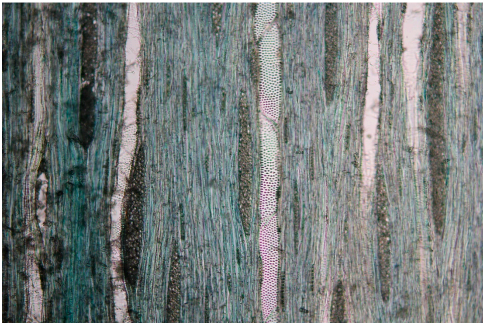
Figure 26. Tangential view of face veneer showing alternate intervessel pitting, spiral thickenings, and cross section of sample perforation plates (100×) that are characteristic of sugar maple ( Acer saccharum ).
