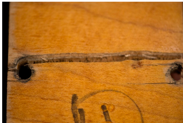
Figure 19. Top View Showing Splitting in Sample 1.
