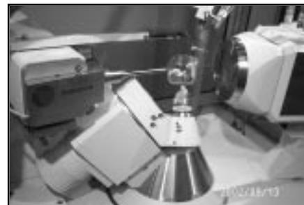
*A diamond-anvil cell mounted on the Xcalibur-2 diffractometer for high-pressure diffraction studies.*
