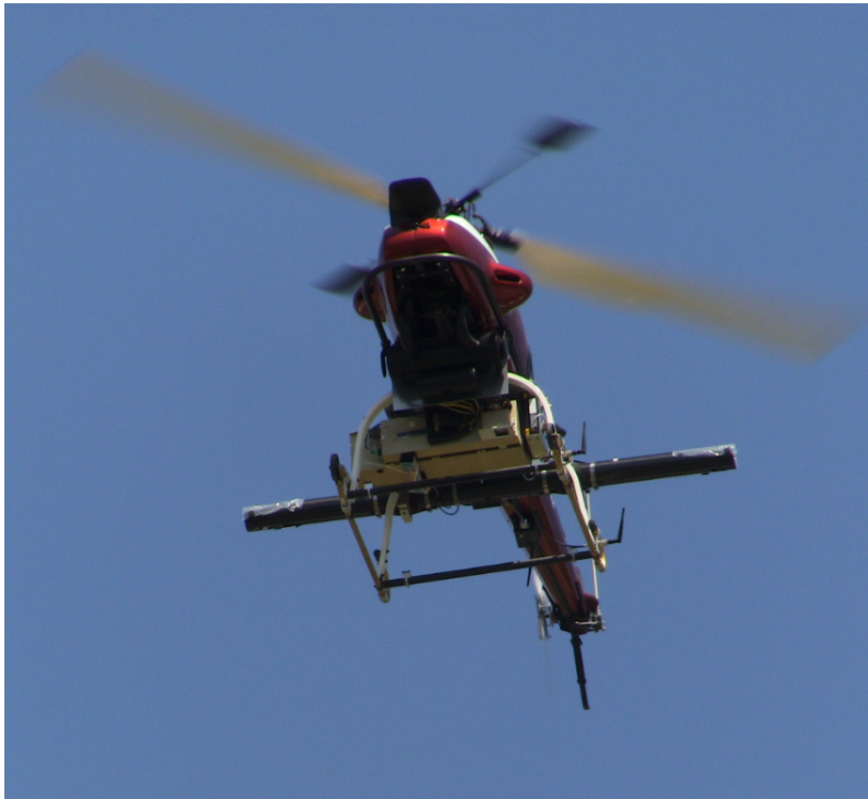
Figure 4.2: The NaI radiation detector and imaging system mounted to the RMAX during one of the missions.
