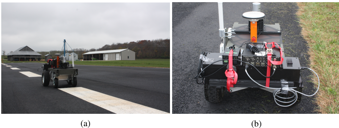
Figure 4.4: (a) The TURTLE at Kentland Farm, Blacksburg, VA where all experiments took place. (b) RSI 701 radiation detector mounted on the back of the TURTLE.
