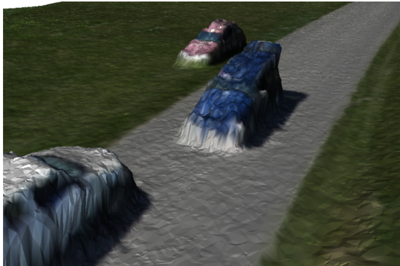
Figure 4.19: A view of the point cloud of Kentland Farm generated using Agisoft that illustrates the level of detail possible using off-the-shelf cameras.
