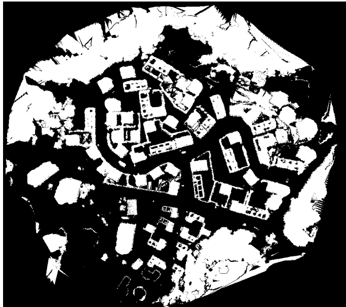
Figure 5.5: Obstacles identified in the scene using the DEM generated by the aerial imagery. By seeding the ground region and iteratively expanding the region, the points in the overhead map not classified as ground are classified as obstacles.
