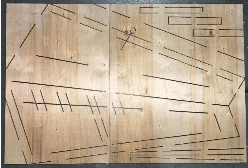
Figure 31. EcoSoar wing template
