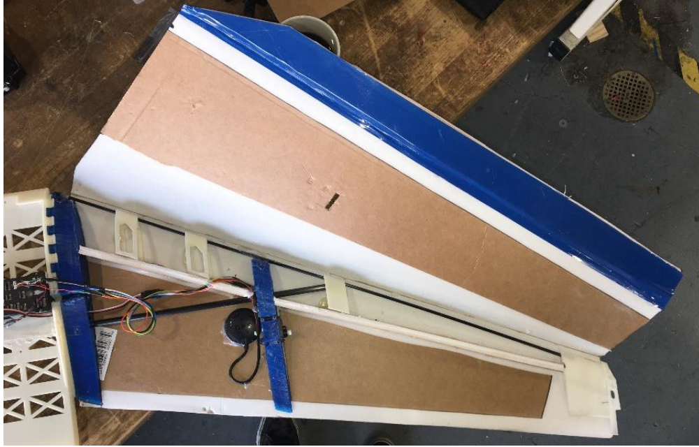
Figure 12. Insides of EcoUV's right wing, showing the new 3D printed components
