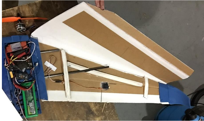
Figure 10. Inside look of “Red,” showing the crafting techniques used to shape the wing
