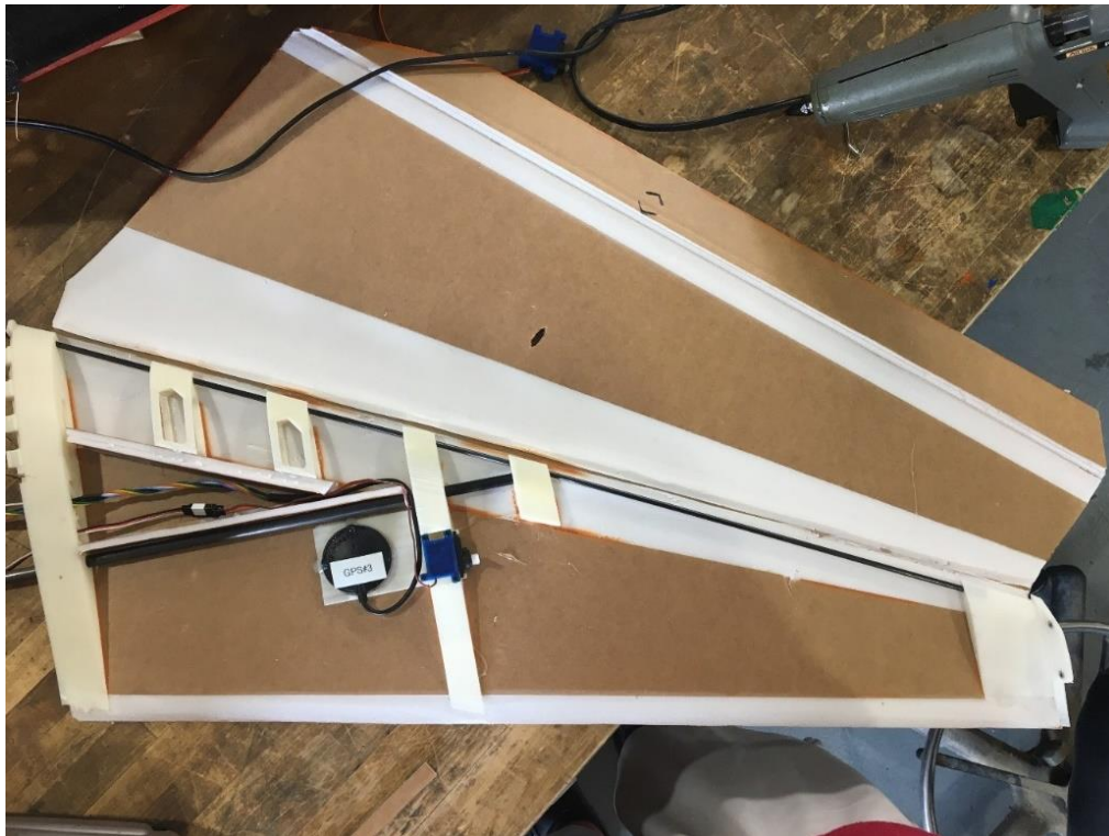
Figure 32. Inside look of EcolR's right wing
