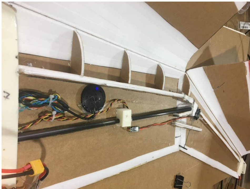
Figure 53. Inside of right wing
