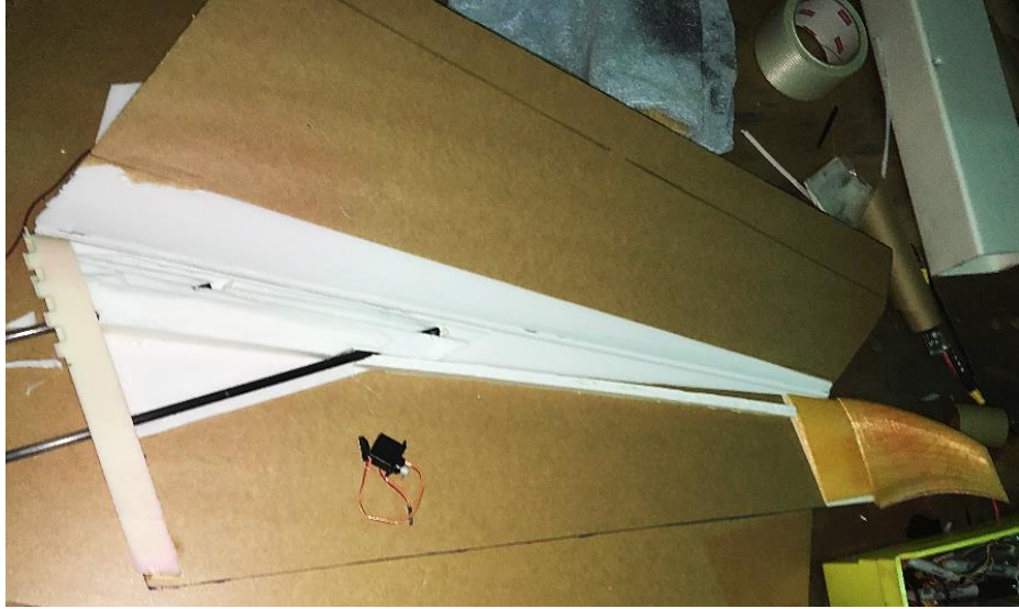
Figure 11. Inside look of incomplete “Green” Foamie, showing the elevated leading edge support used to shape the wing
