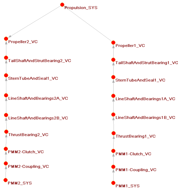
Figure 5 - Mechanical Plex Logical Architecture (A. Brown, Marine Engineering 2018)
