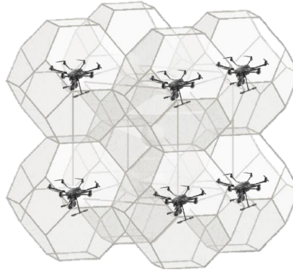
Figure 9.4: Deployment of drone-BSs based on truncated octahedron cells.
