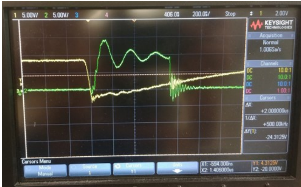
Figure 5.10: Two ferrite beads being used, green trace (top waveform) represents SiC MOS-FET output voltage
