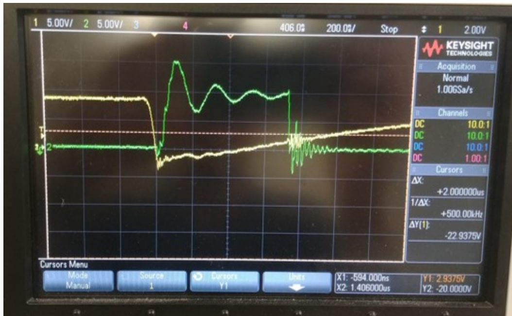
Figure 5.11: Three ferrite beads being used, green trace (top waveform) represents SiC MOSFET output voltage
