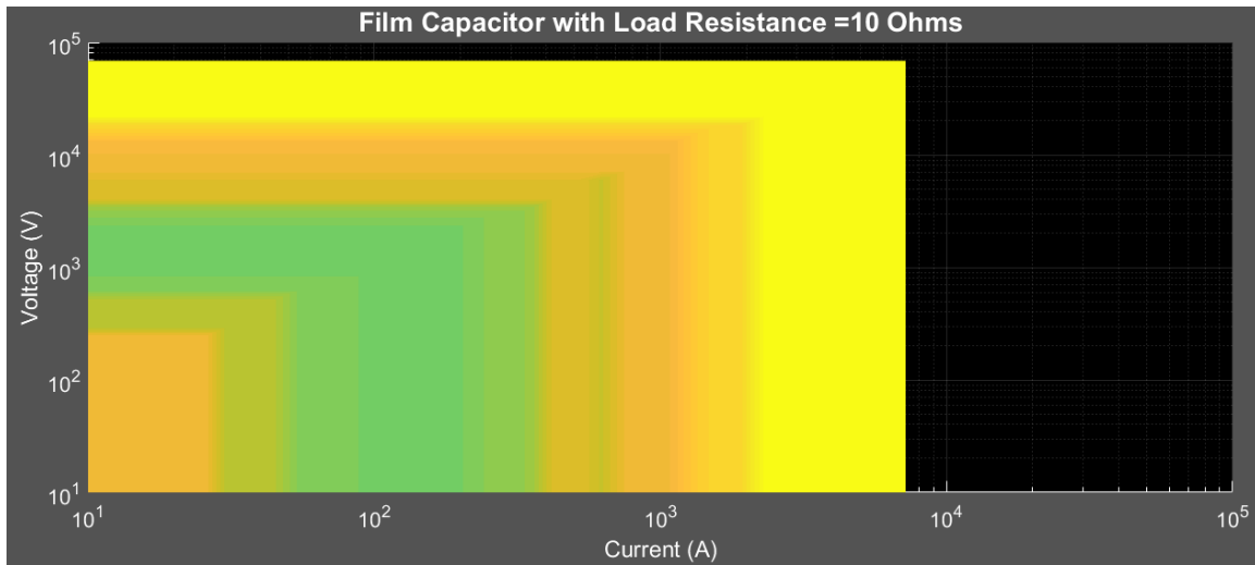
Figure 4.3: Example output of MATLAB algorithm in a surface plot capacitor comparison with coloring representing varying overall LTD costs
