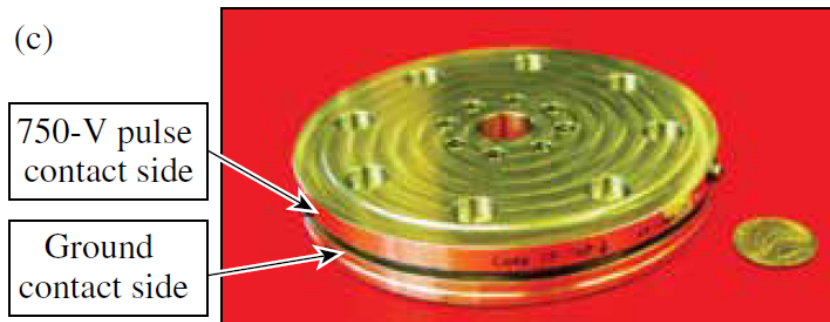
Figure 3.10: LTD transformer design. Image from W. Bittle. Made in 2012. [19]
