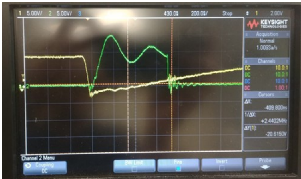
Figure 5.9: One ferrite bead being used, green trace (top waveform) represents SiC MOSFET output voltage
