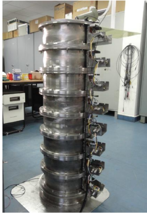
Figure 3.4: Makeup of the 22kV LTD. Image from S.S. Basu. et al. Made in 2014. [17]
