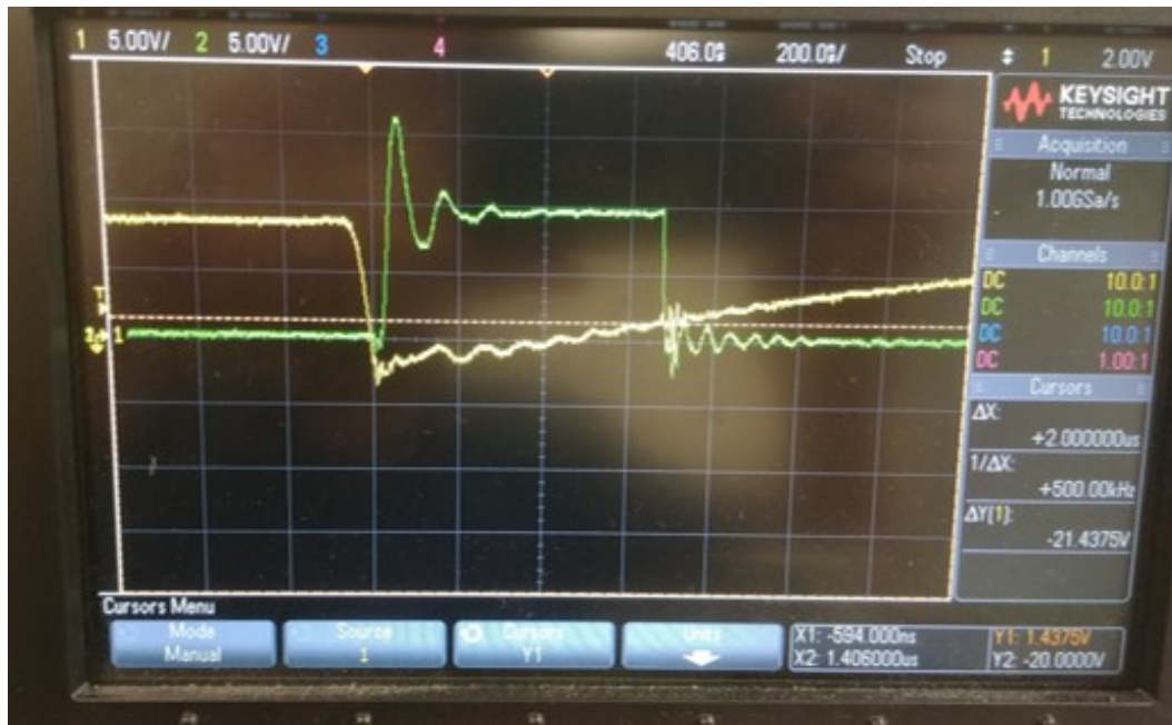
Figure 5.12: Four ferrite beads being used, green trace (top waveform) represents SiC MOSFET output voltage
