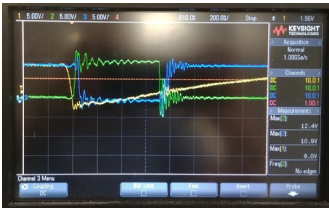
Figure 5.8: Control test using no ferrite beads, green trace line (positive square pulse waveform) represents SiC MOSFET output voltage.
