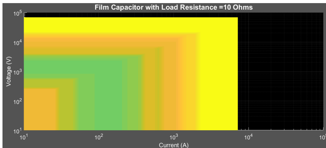
Figure 4: Capacitor surface plot view output from the MATLAB modeling code
