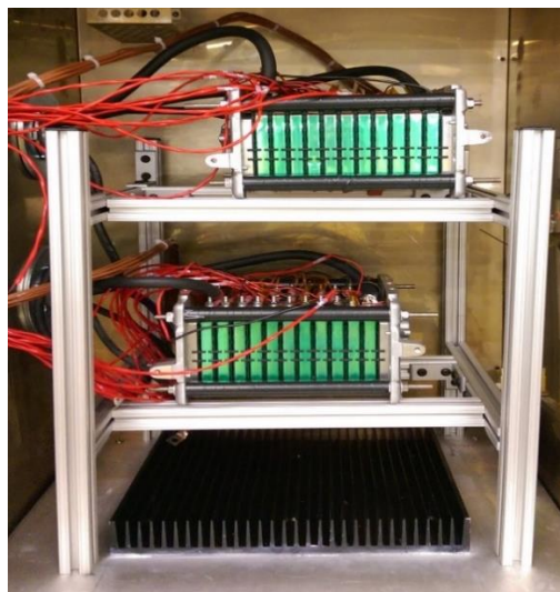
Figure 5: Batteries assembled into two test packs
