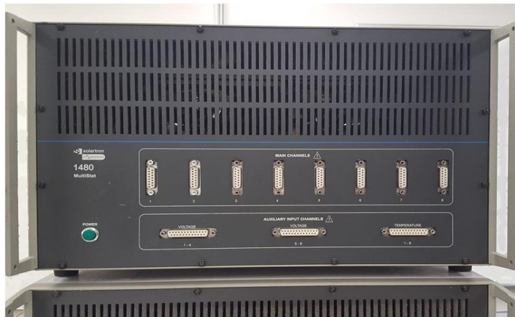
Figure 21: Solatron eight-channel potentiostat used for cycling coin cells
