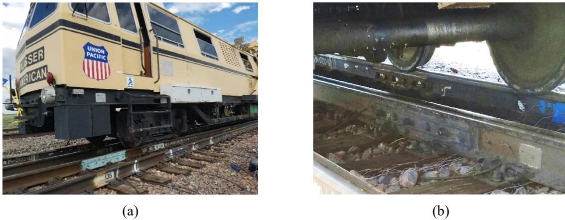
Figure 6.31. In-field loading experiment showing (a) the welder used to load the insulated joint, and (b) the wheels loading the insulated joint and the instrumented rail section used for stress measurements.
