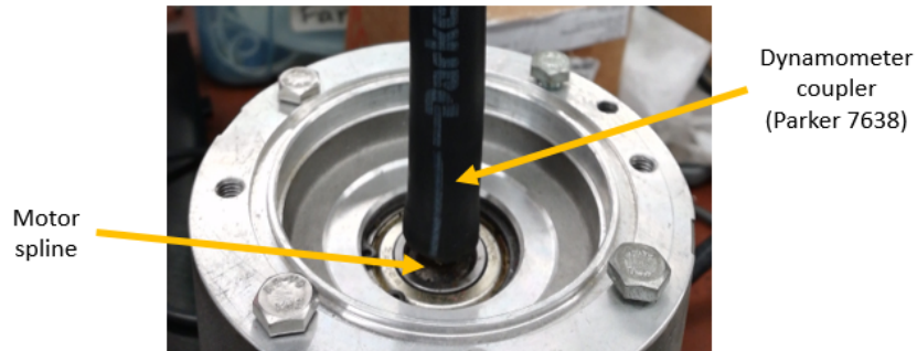
Figure 5-6: Motor spline and dynamometer coupler
