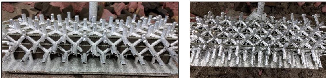
Figure 3-11. Cast parts – Octet cellular structures, before and after sand removal
