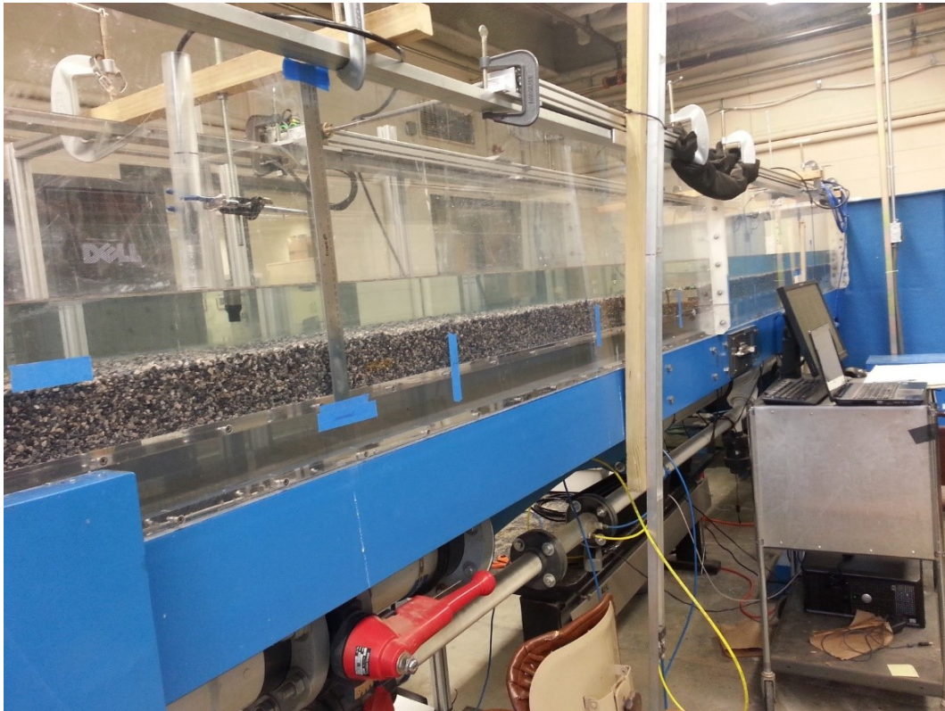
Figure 3.1: Flume channel with unimodal gravel bed. Upstream OBS visible on left.
