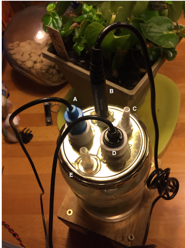
Figure 9: Bioreactor vessel cap assembly, showing probe location. Starting from the blue probe on the bottom left, the probes and connectors shown in the picture are (A) the pH probe; (B) temperature probe; (C) aeration port; (D) DO probe; (E) sampling port. The probes are sealed and secured in place by silicone sealant.
