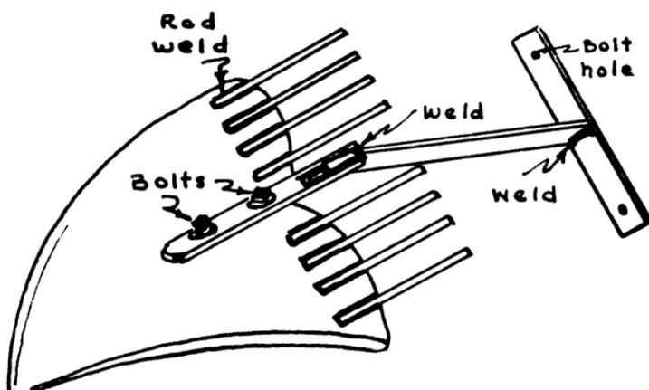
This potato digger is designed for use with a garden tractor and will work very well in any good garden soil. Some skill in shaping iron and in welding is needed but for one used to working with iron, the task should not be difficult.
