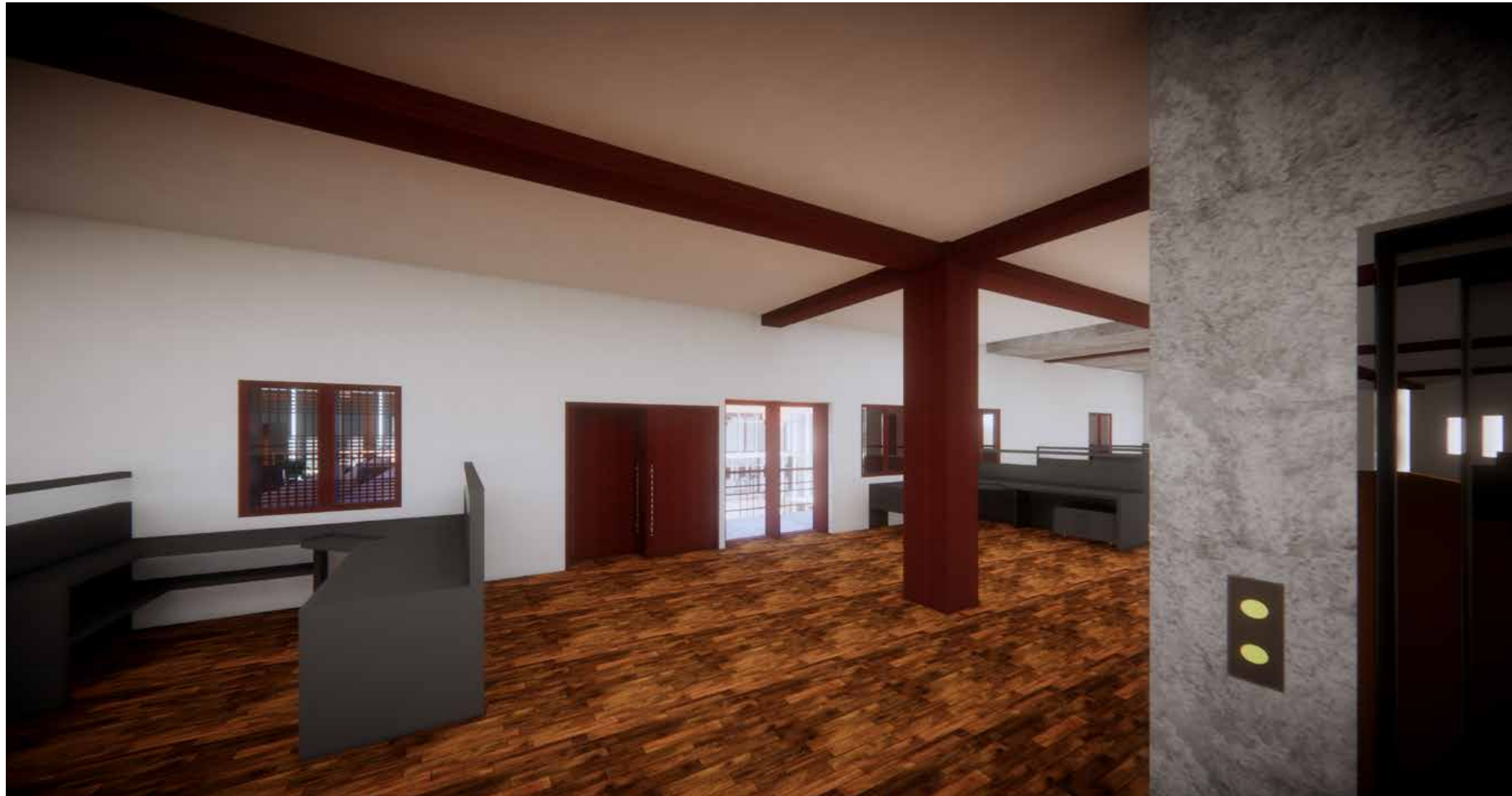
Heavy Timber beams are exposed throughout the design.
