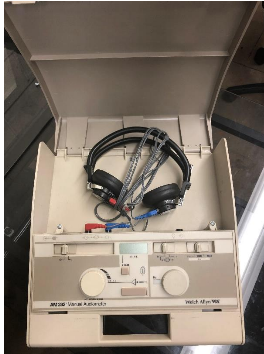
Figure 3.9: Allyn AM 232 Manual Audiometer, which has a set of headphones and a control panel for hearing tests.
