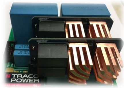
Fig. 5-13 Curved-fin heat sink design for the first-version switching cell
