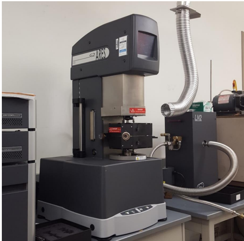
Figure 4.2. Dynamic Mechanical Analyzer used to obtain the rubber properties of the CVTech belt. An oven around the sample allows the temperature dependence of the material properties to be determined.
