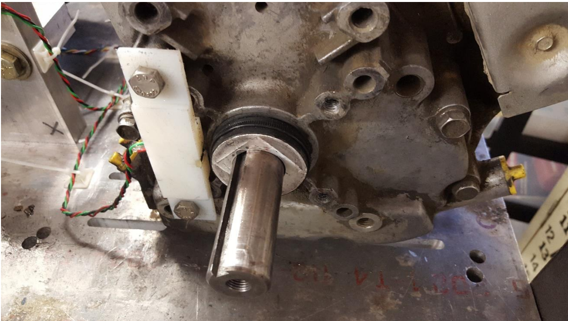
Figure 8.5. Hall Effect sensor used to measure the engine shaft speed. The sensor is embedded in a nylon block that is bolted to the crankcase of the engine. The sensor is encased in epoxy for protection.
