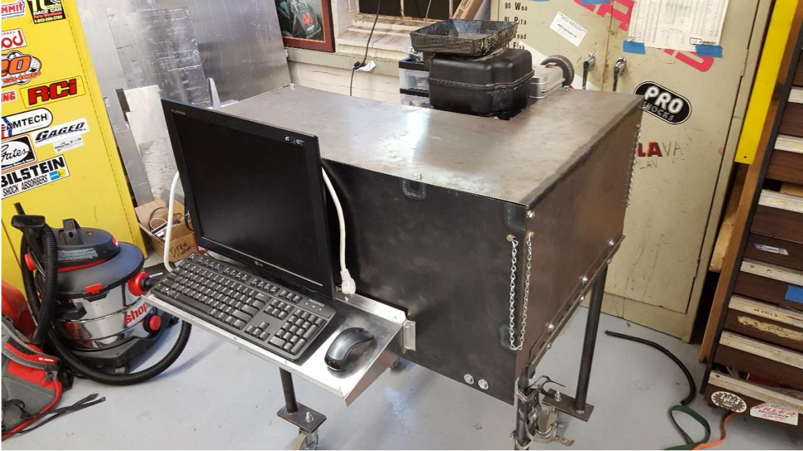
Figure 8.3. Dynamometer with the safety cage closed. An attached monitor and keyboard provide a user interface and allow for the system to be fully contained.
