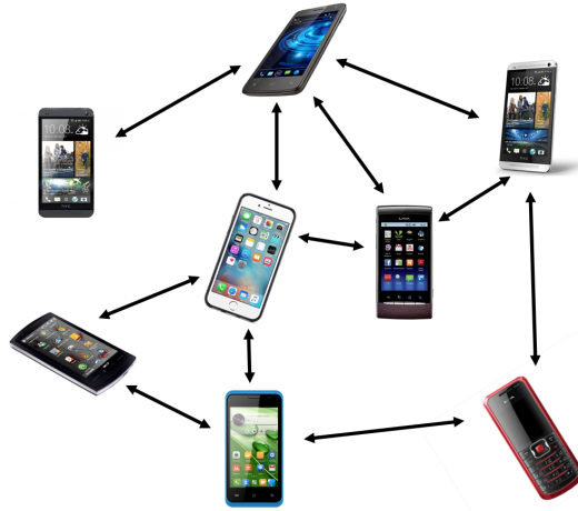
Figure 2.1: Figure depicting ad hoc connections between the mobiles in a MANET
