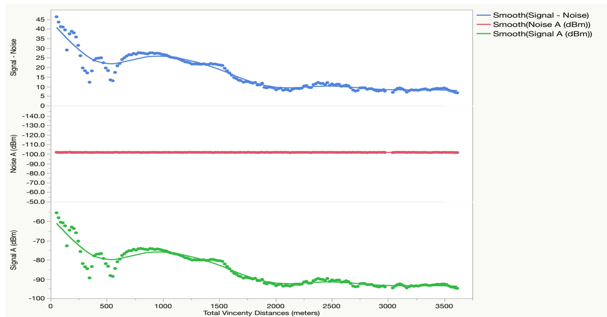
Figure 4-11. The noise was limited and remained constant at the secure testing facility because the staff members implemented a radio silence period during testing.
