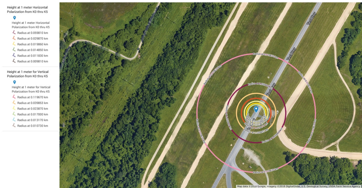
Figure 2-3. Using Google Maps, the horizontal ( d_h^k ) and vertical ( d_v^k ) polarization null points are depicted for K=0 to K=5 with a DSRC RSU height ( h_t ) at 1 meter using Red-Green-Blue color scheme.
