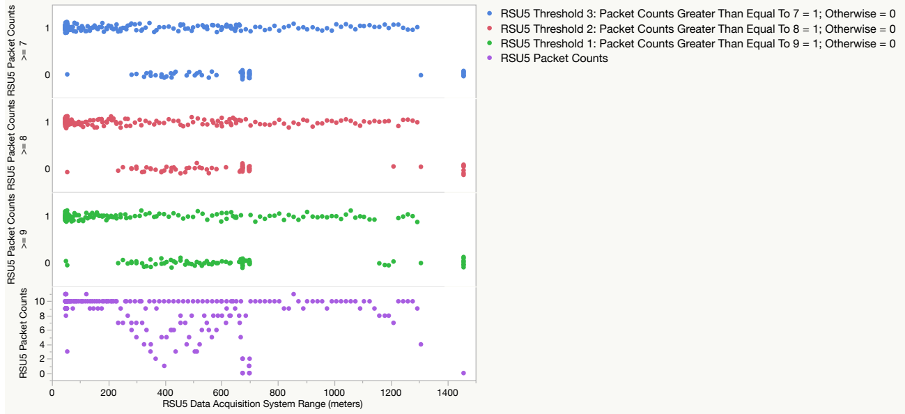
Figure 5-7. The three thresholds for packet counts from DSRC RSU-5
