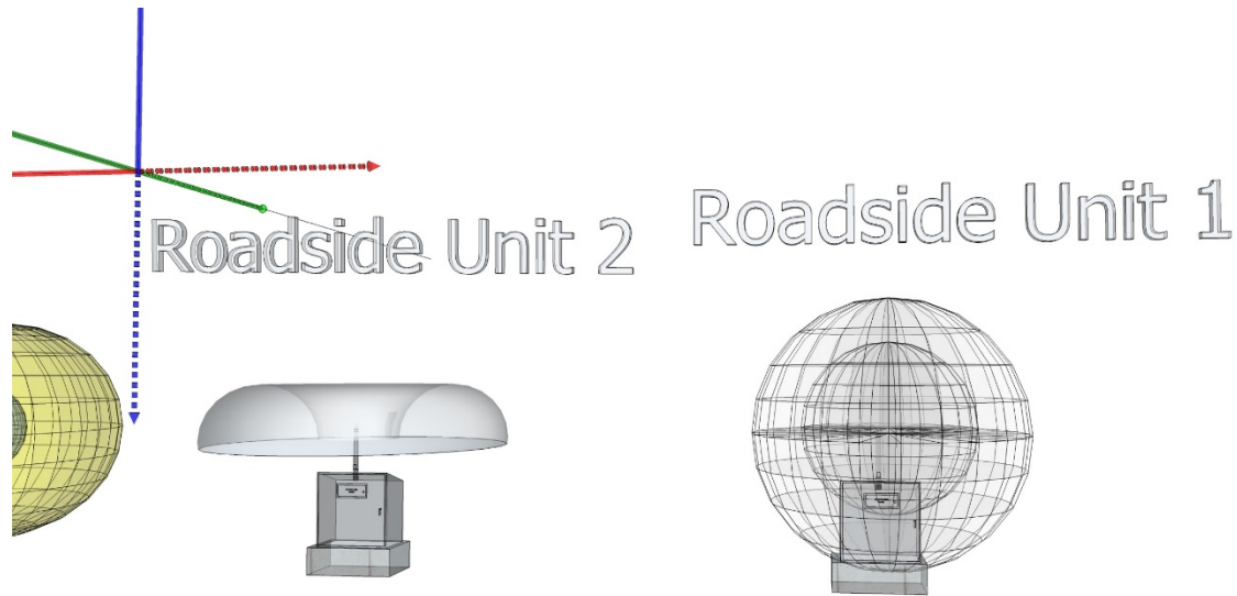
Figure A-6. A 3-dimensional elevation plane pattern with electromagnetic waves along the earth's horizon plane for RSU 1 and RSU 2.
