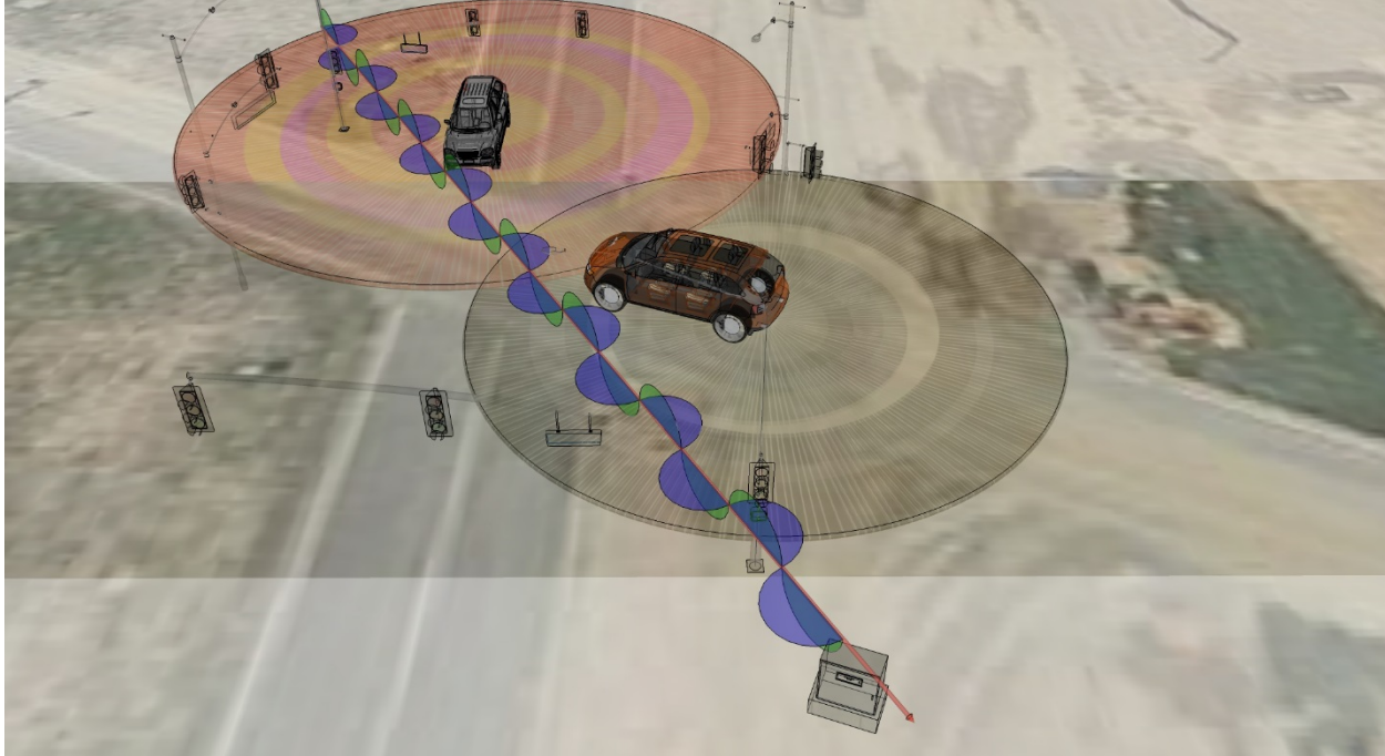
Figure A-1. A RLVW scenario with two approaching vehicles that transmit and receive electromagnetic waves from/to the RSUs.
