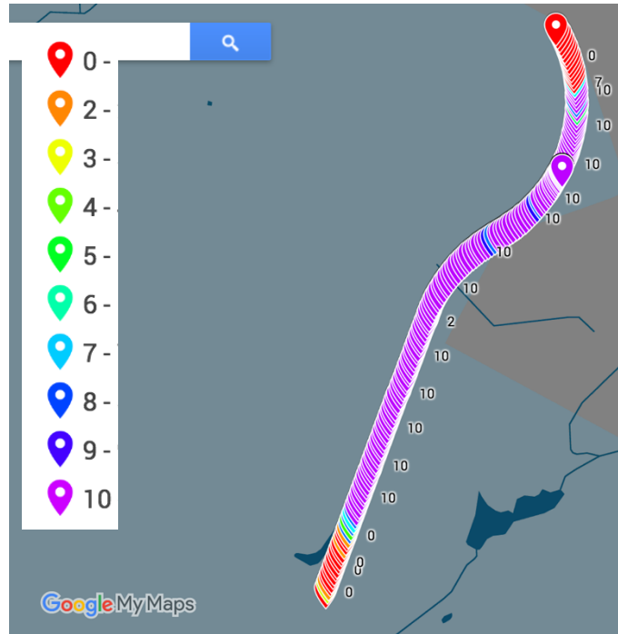
Figure 5-18. Packet counts from RSU-17 around a circular test track using Google My Maps.
