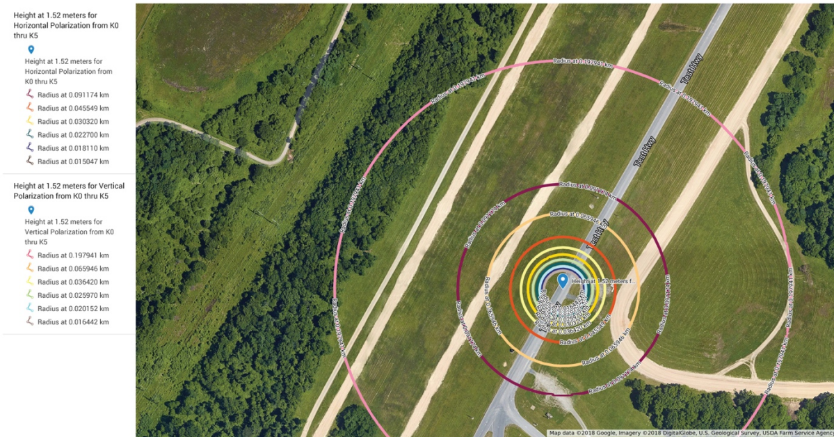
Figure 2-5. Using Google Maps, the horizontal ( d_h^k ) and vertical ( d_v^k ) polarization null points are depicted for K=0 to K=5 with a DSRC RSU height ( h_t ) at 1.524 meters using Red-Green-Blue color scheme.
