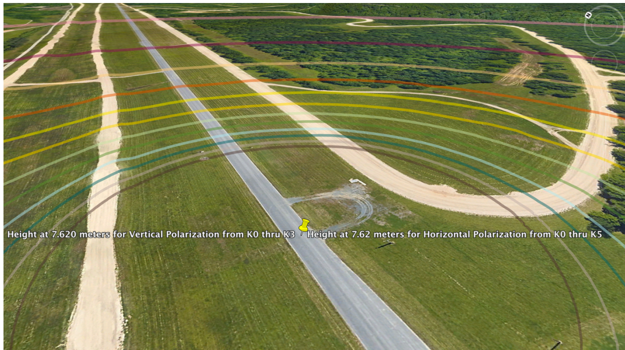
Figure 2-14. Using Google Earth, the horizontal ( d_h^k ) and vertical ( d_v^k ) polarization null points are depicted for K=0 to K=5 with a DSRC RSU height ( h_t ) at 7.620 meters using Red-Green-Blue color scheme.
