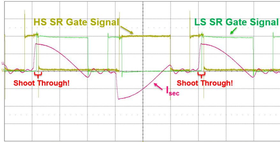
Figure 3.2. SR shoot through from current ringing
