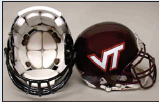
The CIB head impact acceleration measuring system used in Virginia Tech football helmets.
