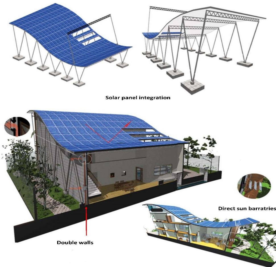
Figure 7-10 Shows the Eco-Friendly House structure and sections including solar panel integration and the house envelope (Aloshan et al. 2009)
