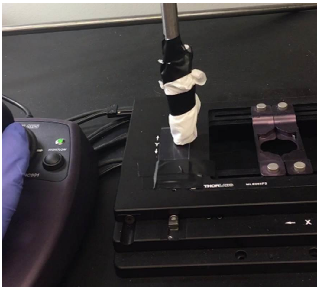
Figure 3.4. Motorized abrasive rod setup for macro-scale scratch testing of films.
