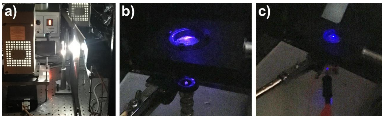
Figure 3.15. Monochromator lamp testing setup. (a) Lamp (left), lens (middle), monochromator (right), monochromator controller (bottom left). (b) Si photodiode with the same circular spot size as on the device with use of a lens. The pinhole cap was removed from the Si photodiode for this calibration. (c) OPV device under monochromator source in plexiglass box. The plexiglass lid was installed for Si photodiode calibration and OPV device testing.
