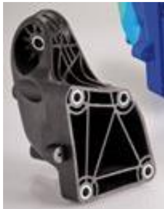
Fig 1.1 Bracket used to secure an engine in a car. Note that the part is not a solid block of material and has narrow supporting beams. The beams and gross shape of the part make using thermosetting materials impossible. FRTs must be used to make this part. [Source: Amanda Jacob, “Daimler replaces aluminium engine support with composite in Mercedes GL class.” 6 Mar 2013. http://www.materialstoday.com/composite-applications/news/daimler-replaces-aluminium-engine-support-with/ ]
