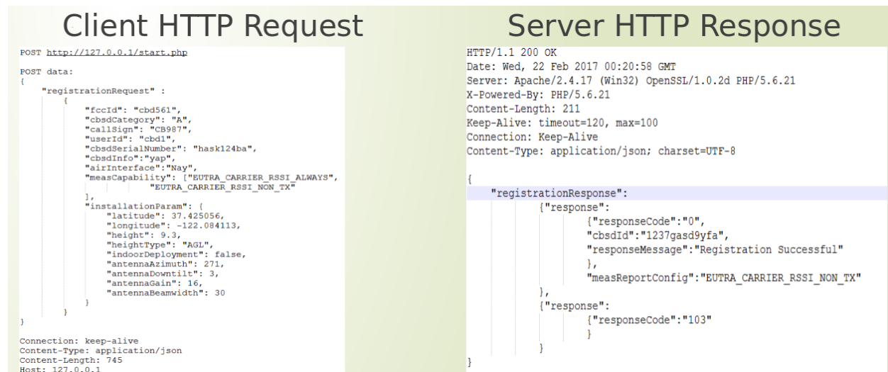
Figure 1.1: Request Reply Response Example between SAS and CBSD
